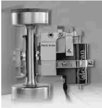
FIGURE 10.11 Extensometer for metal test coupons.
