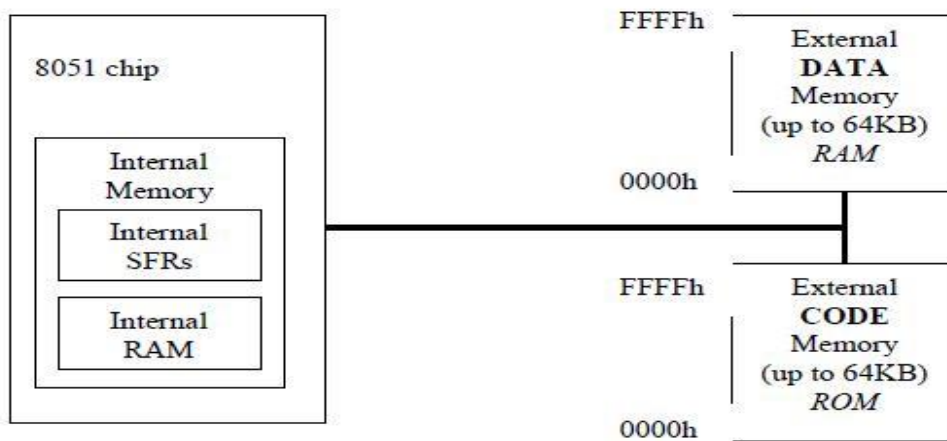
Figure : Memory structure of 8051
