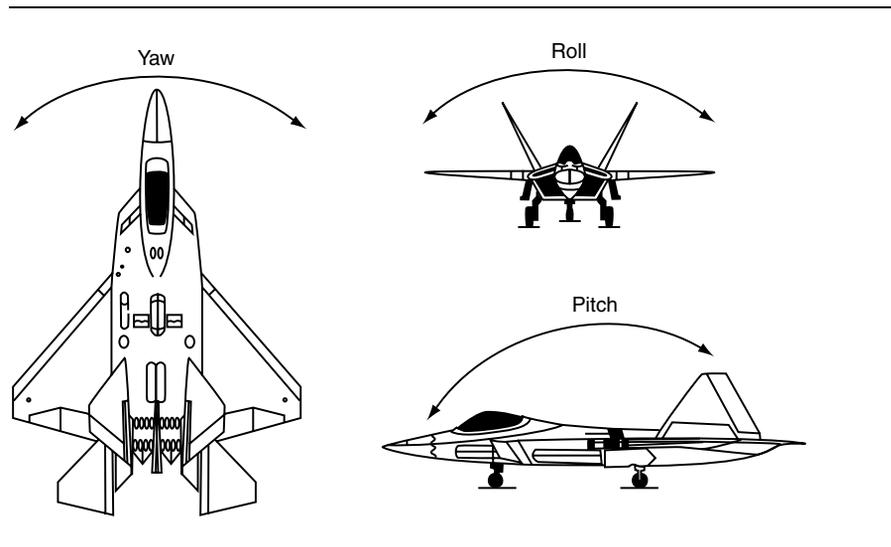
Figure 3.73 Local rotation axes of an aircraft
