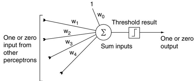
Figure 7.19 Perceptron algorithm
