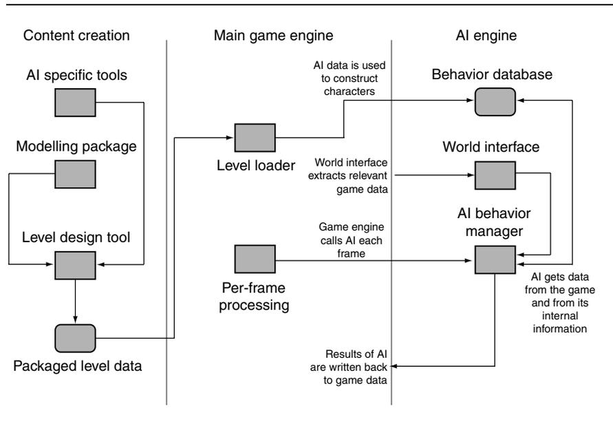
Figure 2.2 AI Schematic
