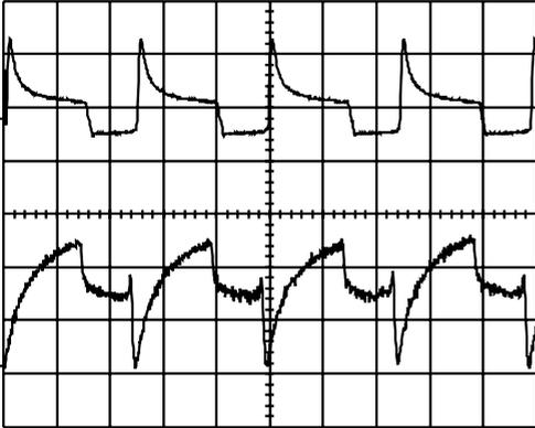
**Figure 5.26** Variation of light output from an uncoated fluorescent lamp. Photodiode at 30 cm from the tube, lightmeter set to range 3. Lower trace: light output as measured by circuit of Figure 5.23, 5 ms/div. horizontal, 0.2 V/div. vertical, 0 V at centreline. Upper trace: waveform of the voltage applied across the tube, via capacitive pick-up, 5 ms/div. horizontal, 2 V/div. vertical, 0 V at two divisions above centreline
