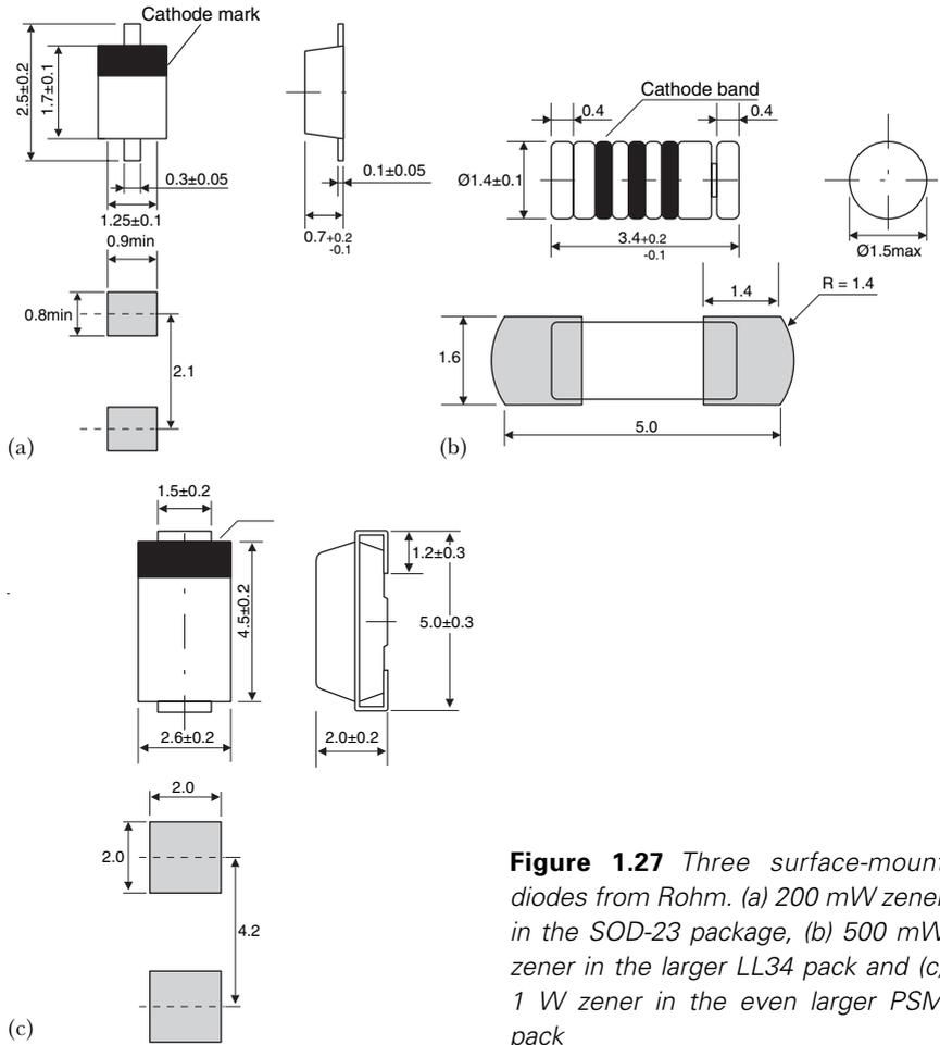
**Figure 1.27** Three surface-mount diodes from Rohm. (a) 200 mW zener in the SOD-23 package, (b) 500 mW zener in the larger LL34 pack and (c) 1 W zener in the even larger PSM pack
