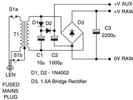
**Figure 6.19** *The necessary raw and auxiliary supplies*
