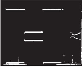
**Figure 6.14** Waveform at MCT gate drive by a 10 kHz squarewave using the UC3705N, double exposure showing both the positive- and negative-going transitions; 10 V/div. vertical, 20 μs/div. switching to 200 ns/div. horizontal
