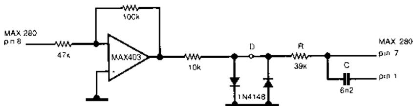
**Figure 3.10** Turning a filter into an oscillator. Feeding the output from the basic filter to its input via an inverting amplifier, using a pair of diodes for amplitude control, gives a good sinewave. Switching the THD meter's bandwidth gives a 'virtually pure' third harmonic
