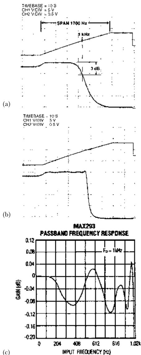
**Figure 3.21** (a) The ramp-voltage applied to the swept frequency oscillator (upper trace) and the detected voltage output from the MAX291 Butterworth 8 pole filter, set to  $F_o = 1$  kHz (lower trace). (b) As (a), but using the MAX293 elliptic filter with its 1.5:1 ratio of  $F_s$  to  $F_o$ . (c) The manufacturer's frequency response data for the MAX293
