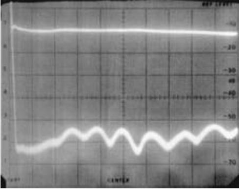
**Figure 4.27** Upper trace as Figure 4.26, for reference. Lower trace, output from port A of the isolator with the input applied to port B. Spectrum analyser settings as for Figure 4.26 except video filter at max.
