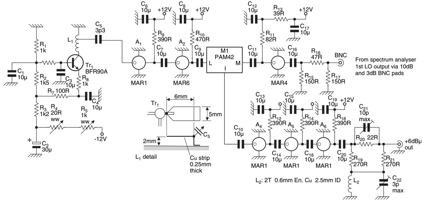
**Figure 4.25** Circuit diagram of an appliqué box for an HP 8558B spectrum analyser, providing a 0–1500 MHz tracking generator output. (Reproduced with permission from *Electronic Product Design*, July 1994, p.17) (Note: for 10 $\mu$  read 10n)
