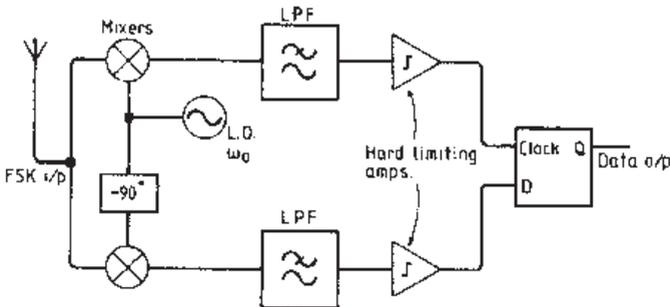
Figure 7.3 Homodyne receiver for frequency-shift keyed transmission
