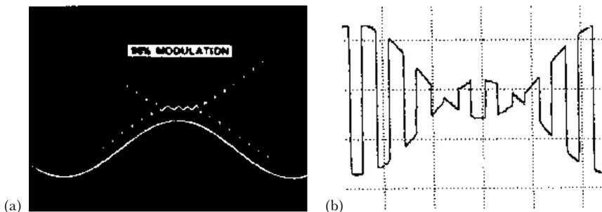
**Figure 7.13** (a) AM with modulation index of 96%. The waveform is continuous with no sudden phase changes. (b) AM with modulation index of 130%; instantaneous 180° phase flips are visible twice per cycle
