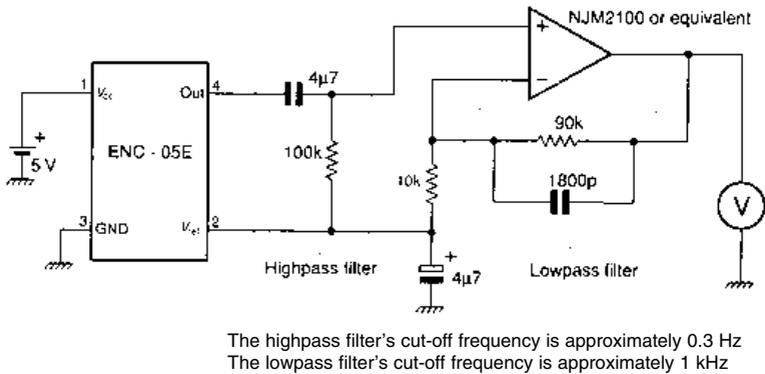
**Figure 2.13** Sample amplifier circuit from the ENC-05E A1 solid state gyro data sheet. (Note that the base diagram shown is confusing;  $V_{ref}$  is actually on the same side of the device as  $V_{cc}$ )
