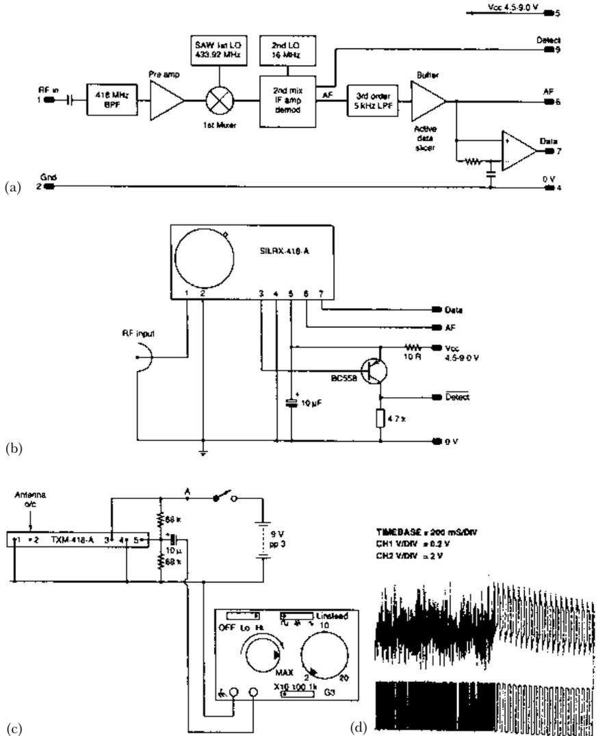
**Figure 7.16** The SILRX-418-A receiver block diagram. (b) Basic receiver test circuit (see text). (c) The transmitter circuit used with (b). (d) The receiver audio (upper trace) and data (lower trace) outputs before and after transmitter switch-on
