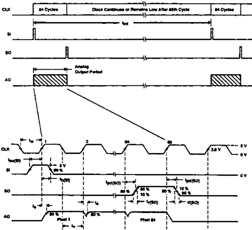
**Figure 5.2** The pixel outputs appear sequentially on the  $A_0$  pin following the rising edges of the next 64 clock pulses that follow the assertion of the SI pulse, assuming its set-up and hold times are met. Following the sample time  $t_s$ , the pixel analog data is valid for at least the period  $t_v$
