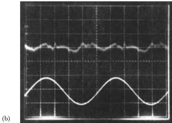
**Figure 3.23** (a) Circuit of a digitally tuned sinewave audio oscillator using the MAX294. (b) The circuit's output at 1 kHz (lower trace) and the residual signal after filtering out the fundamental, representing the total harmonic distortion (upper trace)
