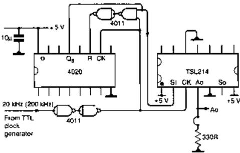
**Figure 5.3** Circuit used for initial investigation of TSL214 operation. An SI (serial input) pulse is produced for every 128th clock pulse. The 64 clock pulses following SI read out the analog light intensity-related signals at pin  $A_0$ .
