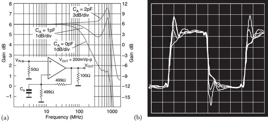
**Figure 4.24** (a) Bandwidth extension for the AD8009 achieved (for a gain of +2) by adding capacitance from the inverting input to ground. (b) The effect of these three values of capacitance on the pulse response
