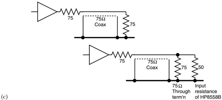
**Figure 3.33** (a) Test circuit used to produce a 5 MHz squarewave with fast edges, to test the probe of Figure 3.31. The 27  $\Omega$  plus 330 pF snubber at the output suppressed ringing on the test waveform. (b) Test set-up used to test the wideband probe of Figure 3.32. (c) Showing how the 6 dB signal reduction in normal use becomes 11 dB in the test set-up of (b) above. Together with the 10 dB pad at the sweeper output, this accounts for the 21 dB separation of the traces in Figure 3.32(b)
