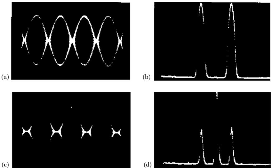
**Figure 7.12** (a) Double sideband suppressed carrier output of the MC1496. (b) Spectrum of (a),  $rf = 0.5$  MHz, baseband modulation 1 kHz. (c) 100% modulation AM, also with  $rf = 0.5$  MHz, baseband modulation 1 kHz. (d) Spectrum of (c)
