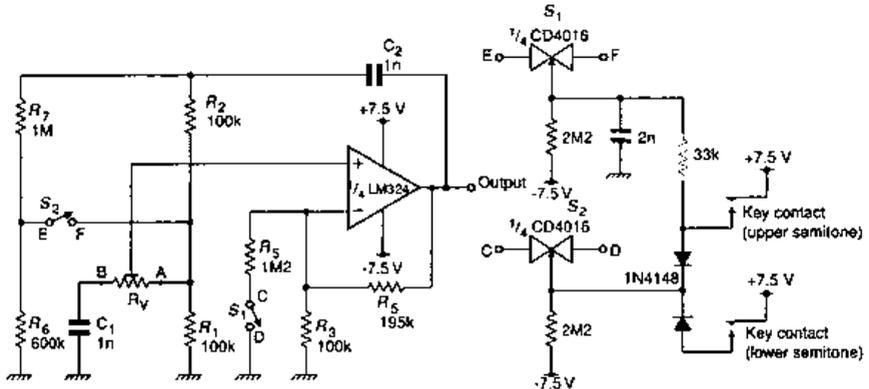
**Figure 2.10** The circuit modified to sound either of two adjacent semitones, according to which key is pressed. The addition of both  $R_6$  and  $R_7$  keeps the loop gain the same when  $S_2$  is closed, leaving the amount of clipping at the rails the same for either semitone (see Figure 2.11(a))
