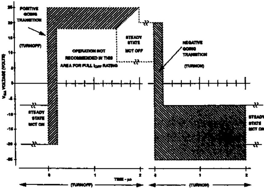
Figure 6.12 Recommended boundary limits for MCT gate waveform
