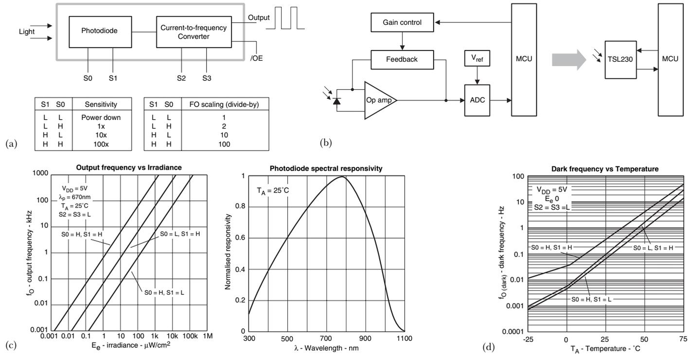
**Figure 5.22** (a) Functional block diagram of the TSL230 programmable light-to-frequency converter. (b) Illustrating the system simplification possible with the TSL230 programmable light-to-frequency converter. (c) Illustrating the various sensitivity ranges available to the user with the TSL230, left, together with spectral responsivity, right. (d) Showing the very low dark frequency output of the TSL230, as a function of temperature
