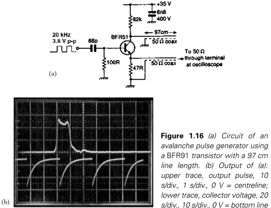
**Figure 1.16** (a) Circuit of an avalanche pulse generator using a BFR91 transistor with a 97 cm line length. (b) Output of (a): upper trace, output pulse, 10 ns/div., 2 V/div., 0 V = centreline; lower trace, collector voltage, 20  $\mu$ s/div., 10 V/div., 0 V = bottom line
