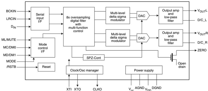
**Figure 1.35** The PCM1717E DAC from Burr-Brown accepts 16 or 18 bit serial data, and provides L and R stereo output channels. With numerous facilities, aimed at CD systems, MPEG audio, MIDI applications, etc.
