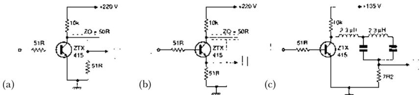
**Figure 1.14** *Circuits producing square output pulses; (a) negative-going output pulses and (b) positive-going pulses both using coaxial lines; (c) negative-going pulses using a lumped component delay line*
