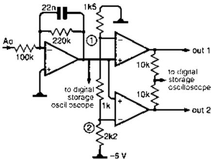
**Figure 5.5** An inverting leaky integrator produces a negative output voltage proportional to the number of pixels which are uncovered. Comparators indicate whether about half the device is illuminated, or more, or less
