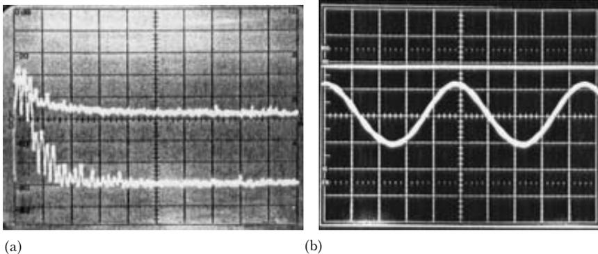
**Figure 7.39** (a) Spectrum analyser sweep, 0–5 kHz, reference level (top of screen) –60 dB, 10 dB/div. vertical, IF bandwidth 30 Hz, smoothing maximum, 100 seconds per division sweep speed. Lower trace, with + and –15 V supplies off. Upper trace, supplies on, circuit as in Figure 7.37. (b) Oscilloscope traces; horizontal, 20 ns/div. Upper trace,  $IC_3$  pin 12, 5 V/div., 0 V at centreline, with coax cable disconnected. Lower trace,  $IC_3$  pin 4, 50 mV/div. ac coupled, coax cable connected
