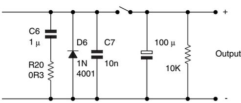
**Figure 6.26** When the separate output switch is closed, the 100  $\mu\text{F}$  capacitor causes the output voltage momentarily to collapse (almost) to zero. The output voltage then ramps up with the PSU in current limit, until the preset voltage is reached, or until the limited available current is drawn through a fault in the circuit under test
