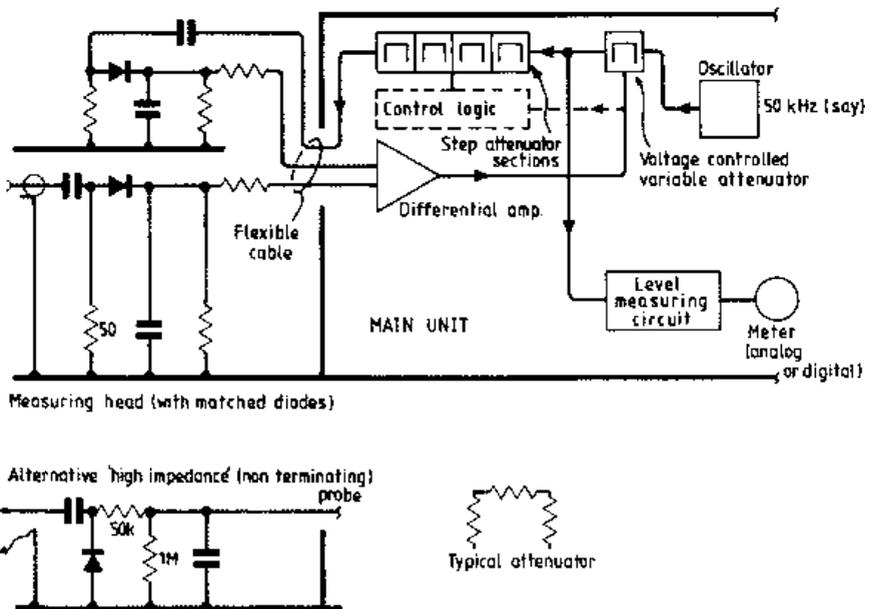
**Figure 4.3** Accurate rf level measurement requires linearisation of the diode response. This can be done by using a dummy diode and separate rf reference source for comparison with the rectified level of the signal under test
