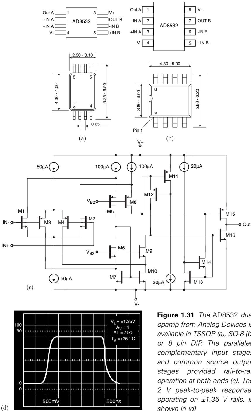
**Figure 1.31** The AD8532 dual opamp from Analog Devices is available in TSSOP (a), SO-8 (b) or 8 pin DIP. The paralleled complementary input stages and common source output stages provided rail-to-rail operation at both ends (c). The 2 V peak-to-peak response, operating on  $\pm 1.35 V$  rails, is shown in (d)
