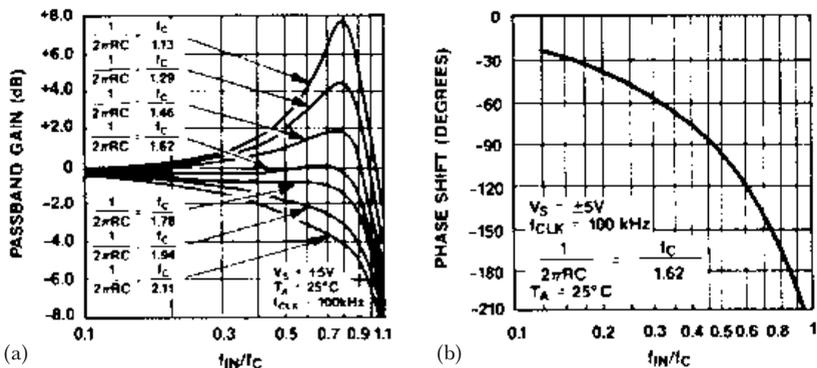
**Figure 3.6** Typical operating characteristics: (a) passband gains versus input frequency; (b) phase shift showing that this characteristic has already reached  $180^\circ$  at 0.85 of the 3 dB cut-off frequency  $f_c$
