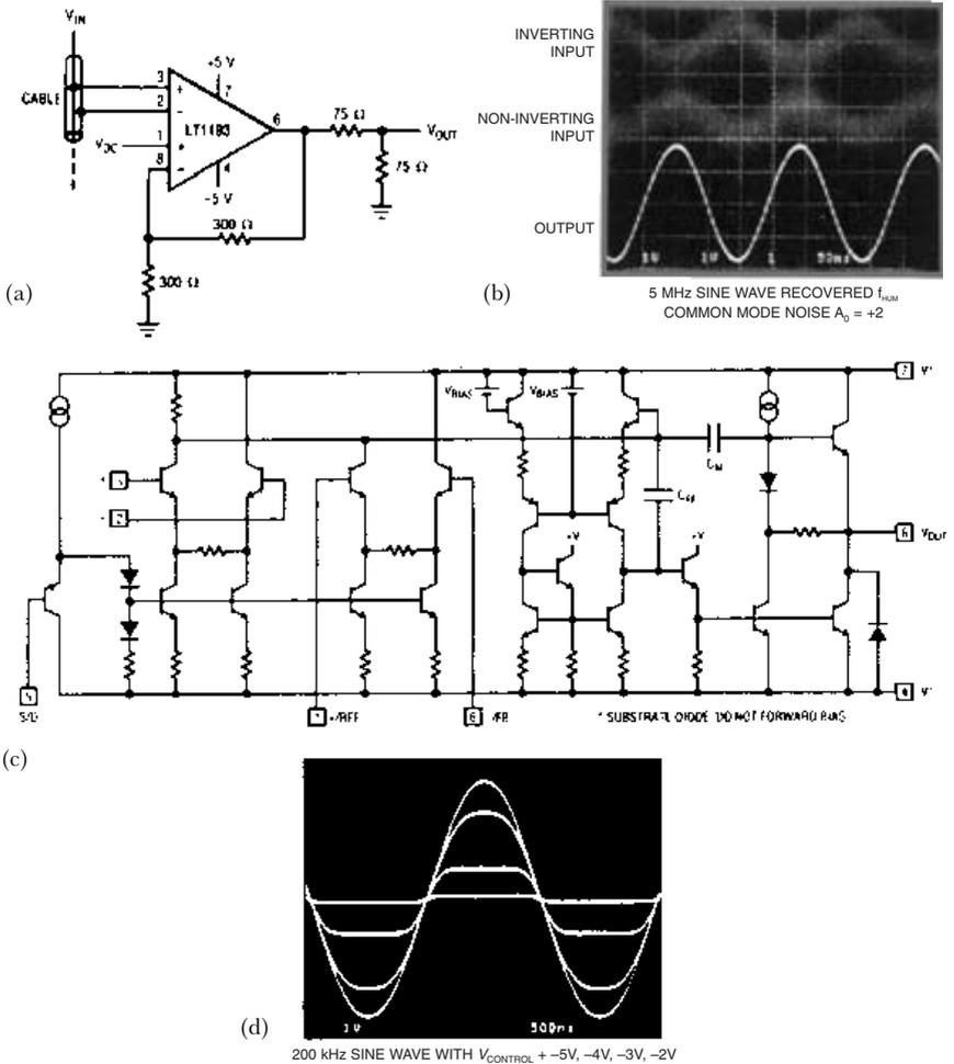
**Figure 3.3** (a) Cable sense amplifier for loop through connections with dc adjust. (b) Recovered signal from common mode noise. (c) LT1193 simplified schematic. (d) Sinewave reduced by limiting the LT1193
