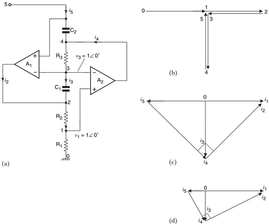
**Figure 1.20** (a) *FDNR* circuit diagram. If  $v_1$  is the voltage at node 1, etc., then  $v_1 = v_3 = v_5$ . Also,  $i_1 = i_2 = i_3$  and  $i_3 = i_4 + i_5$ . (b) Voltage vector diagram for (a) when  $R_1 = R_2 = R_3 = R$ ,  $C_1 = C_2 = C$  and  $f = \frac{1}{2\pi CR}$ . (c) Current vector diagram for (a), for the same conditions as (b). (d) As (c) but for  $f = \frac{1}{4\pi CR}$ . Note that  $i_2$  and  $i_4$  are always in quadrature.
