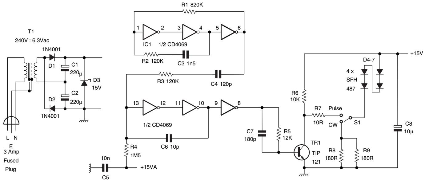
**Figure 5.32** Circuit diagram of a high power IR source, with choice of steady or pulsed output
