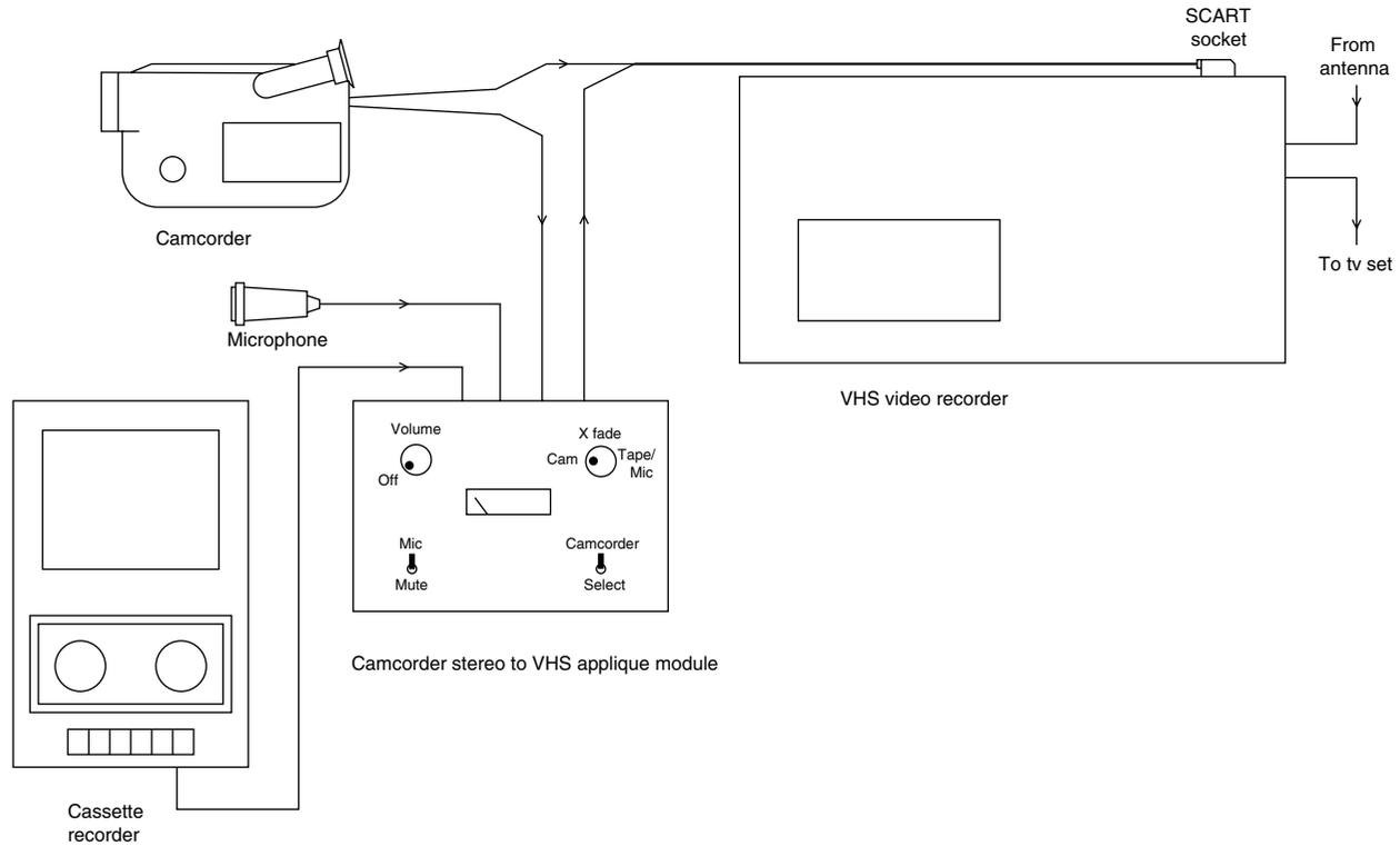
**Figure 2.26** Showing the various pieces of kit interconnected. The sound from the camcorder is routed via the appliqué box. The latter permits cross-fading of the camcorder sound output with sound from tape and/or microphone
