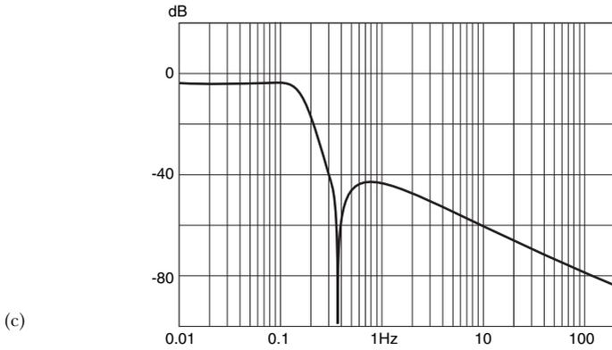
**Figure 1.21** A low component count elliptic lowpass filter with a minimum attenuation of 36 dB from twice the cut-off frequency upwards, the price being as much as 1 dB passband ripple. The minimum capacitor design of (a) is more convenient than (b) for conversion to an FDNR filter. (c) The frequency response of the filter
