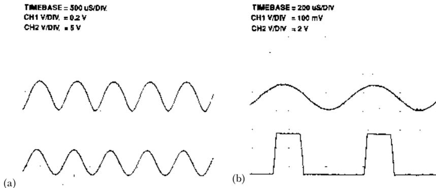
**Figure 7.18** (a) The TXM-UHF and SILRX-418-A can handle linear signals, with some distortion; 1 kHz full amplitude sinewave modulation applied to TX module (lower trace) and as recovered by the receiver (upper trace). (b) At a reduced modulation level (upper trace) the distortion of the received signal is negligible, although the effect of a reduced level into the data slicer is evident (lower trace)
