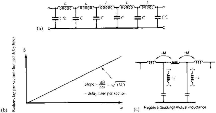
**Figure 1.2** (a) Basic delay line – (b) providing a delay of  $\sqrt{LC}$  seconds per section at dc and low frequencies. (c) Connection of negative inductance in the shunt arms to linearise the group delay over a larger proportion of the filter's passband. Not a physical component, it is implemented by negative mutual inductance (bucking coupling) between sections of series inductance
