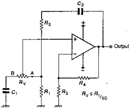
**Figure 2.6** The addition of trimmer potentiometer  $R_V$  permits tuning of the oscillator without changing the attenuation via the Wien network, provided the resistance of the pot's track does not exceed one-tenth of the reactance of  $C_1$
