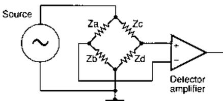
**Figure 3.12** Bridge null detector is a testing application for a differential input amplifier. Both inputs must be very high impedance; additionally, the amplifier requires a high CMRR of around 60 dB for a 1% bridge accuracy
