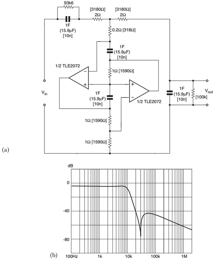
**Figure 1.24** (a) Complete FDNR filter with 10 kHz cut-off frequency. The (values) are a little impractical, but are easily scaled to more sensible [values]. (b) Computed frequency response of the above filter. The cut-off frequency (at  $-1$  dB) is a shade below the intended value, as was that in Figure 1.21(c)
