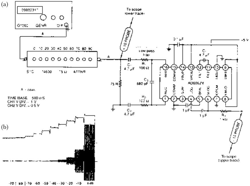
**Figure 1.8** (a) Circuit used to view the log operation at low frequency; (b) input signal (lower trace), increasing in 10 dB steps and the corresponding VLOG output (upper trace). The dip at the end of each 10 dB step is due to the momentary interruption of the signal as the attenuator setting is reduced by 10 dB and the following overshoot to the settling of the Sallen and Key filter
