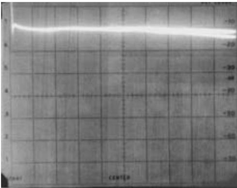
**Figure 4.26** *Upper trace, output of the tracking generator, attenuated by 20 dB. Lower trace, as upper trace, but with the signal routed via port B to port C of the isolator. Reference level –2.5 dB, 10 dB/div., span 0–500 MHz, IF bandwidth 3 MHz, video filter medium*
