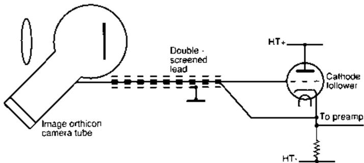
**Figure 3.11** An early application of bootstrapping. The camera signal is connected to its preamplifier via double-screened cable, the inner screen of which is driven by the output of the cathode follower buffer stage. Since the gain of the latter is very nearly unity, there is no ac voltage difference between the inner conductor and the inner of the two screens, so the signal does not 'see' any cable capacitance to ground
