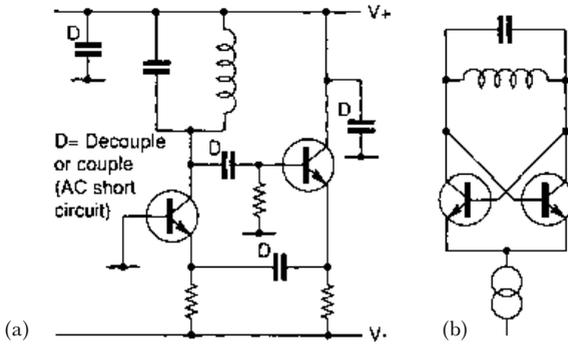
**Figure 4.8** (a) Two transistor oscillator looks at first sight like an emitter follower driving a grounded base stage. But the earth point is an arbitrary convention. (b) If the decoupling capacitors in (a) are shown as short-circuits at rf, the circuit is seen to be a balanced push-pull oscillator
