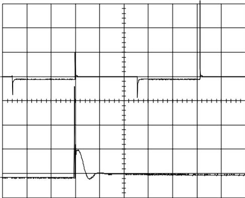
**Figure 6.24** Transient response of the PSU when the load switches between  $1\ \text{A}$  and  $2\ \text{A}$ : upper trace  $500\ \text{mV/div.}$ ,  $200\ \mu\text{s/div.}$ ; lower trace  $500\ \text{mV/div.}$ ,  $5\ \mu\text{s/div.}$
