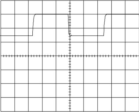
**Figure 6.23** Load switching between  $33\ \Omega$  and  $17.5\ \Omega$ , with the demanded output voltage set to  $15\ \text{V}$  but the current limit reduced to roughly  $0.5\ \text{A}$ , i.e. such that at  $17.5\ \Omega$  the voltage collapses to  $7.5\ \text{V}$ :  $5\ \text{V/div.}$ , centreline =  $0\ \text{V}$ ,  $200\ \mu\text{s/div.}$
