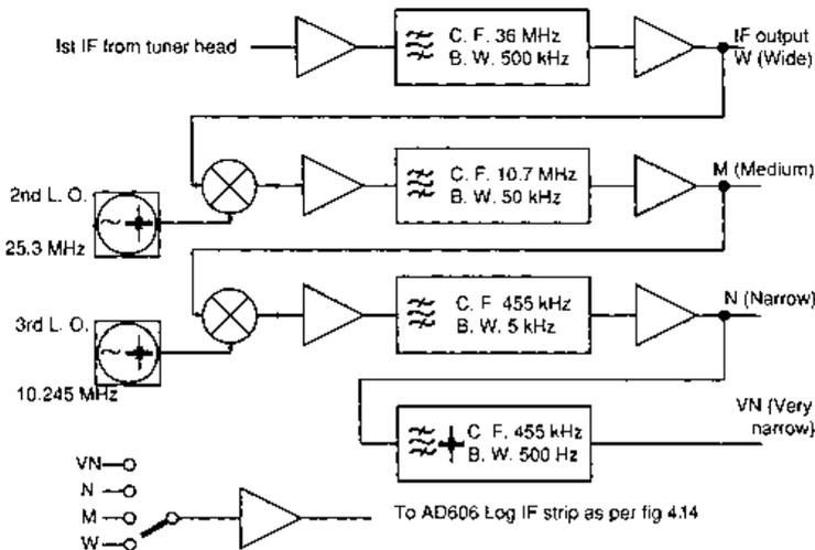
**Figure 4.18** Block diagram showing modified architecture giving a choice of IF bandwidths. It is simpler to provide different signal paths for the different bandwidths rather than select the bandwidth by switching in one or other of several filters all operating at the same IF frequency
