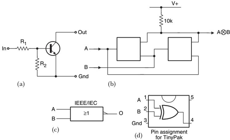
**Figure 1.37** Digital transistors, (a), from Rohm, are available in SOT23 packs (Figure 1.29), with a variety of values for  $R_1$  and  $R_2$ . Two such transistors connected as in (b) give the inverse EXOR or exclusive NOR function. A single component solution is also possible, being readily available in CMOS as the NC7S86M5, (c) and (d), from National Semiconductor
