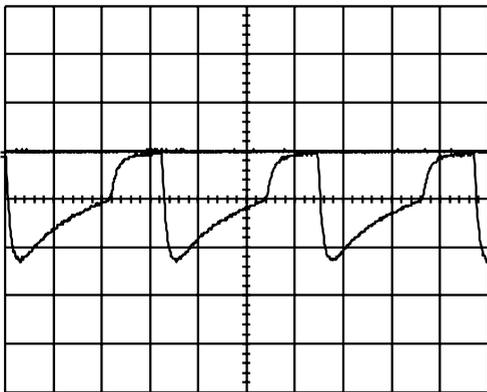
**Figure 5.34** Light output of the circuit of Figure 5.27, measured using range 2 of the lightmeter, at an increased range. 500 mV/div. vertical, 0 V reference line at one division above centreline, 10  $\mu$ s/div. horizontal
