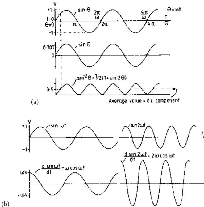
**Figure 7.6** Effects of squaring and differentiating sine waves. Squaring the wave, as in (a), doubles its frequency and produces a dc component. Differentiating, shown in (b), gives a cosine wave with an amplitude proportional to frequency
