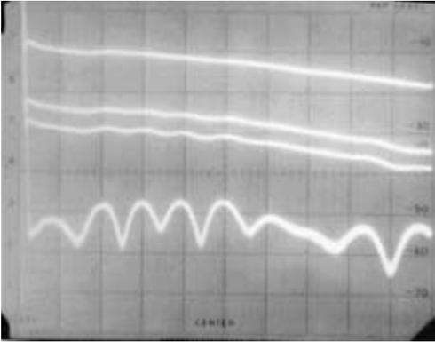
**Figure 4.28** *Traces showing the signal at port C for various degrees of intentional mismatch at port B: with (top to bottom) return loss of 0, 14, 20 and 74 dB. Signal applied to port A as in Figure 4.26, upper trace. Spectrum analyser settings as for Figure 4.27*
