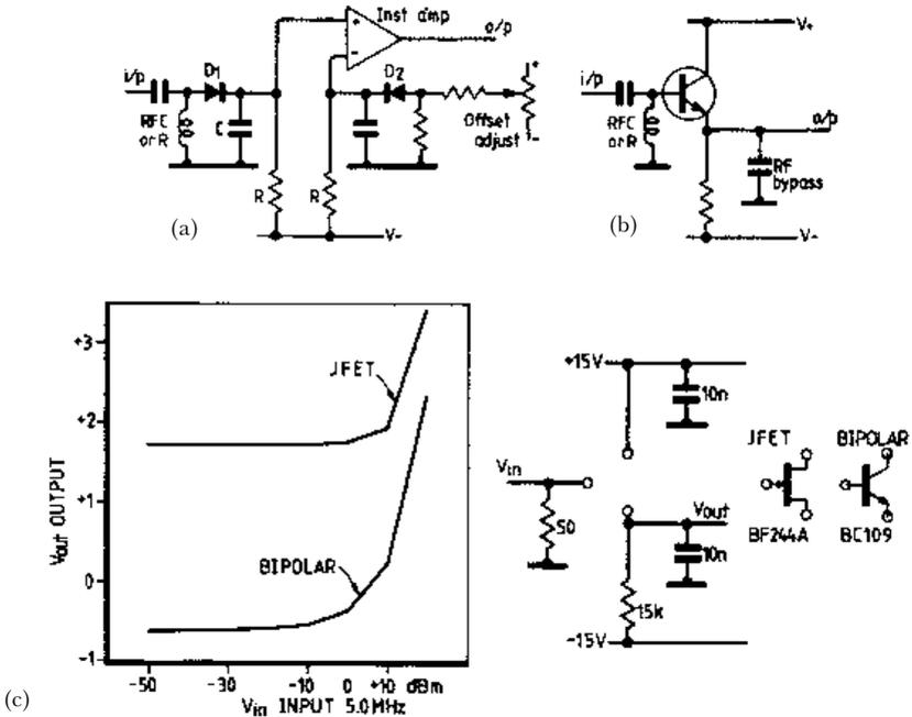
**Figure 4.4** (a) DC bias to the diode improves linearity by several dB. If  $R$  is made high enough, it becomes a current source greatly extending the linear detection region but this also requires a larger negative rail voltage. (b) Functional equivalent of the diode circuit (a). (c) Comparing the performance of a JFET versus bipolar infinite impedance detector. The latter has a more abrupt cut-off providing a higher dynamic range
