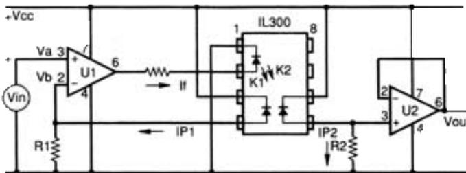
**Figure 5.10** Typical application circuit for the *IL300* linear optocoupler, in positive-going unipolar photoconductive model. Although  $K_1$  and  $K_2$  vary with temperature, their ratio  $K_3$  is virtually temperature independent. Devices are coded into bands according to the spreads of  $K_1$  and  $K_3$
