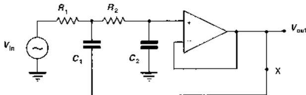
**Figure 2.18** The Sallen and Key second-order lowpass active filter. Cut-off ('corner') frequency is given by  $f_o = 1/(2\pi C_1 C_2 R_1 R_2)$  and  $Q = 1/2 \sqrt{C_1/C_2}$  and dissipation  $D = 1/Q$ . For a maximally flat amplitude (Butterworth) design,  $D = 1.414$ , so  $C_1 = 2C_2$ . The Butterworth design exhibits no peak, and is just 3 dB down at the corner frequency
