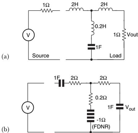
**Figure 1.22** FDNR version of the lowpass filter
