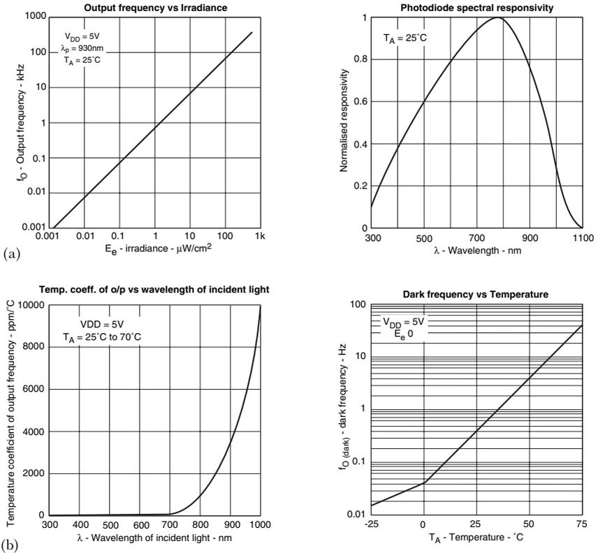
**Figure 5.21** (a) Output frequency versus incident illumination, left, and spectral response, right, for the TSL235 light-to-frequency converter. (b) Temperature coefficient of output frequency of the TSL235, as a function of wavelength, left, and dark frequency performance, right
