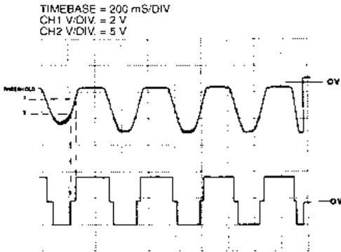
**Figure 5.6** Operating the device in the analog system of Figure 5.5 – 330R load resistor shown in Figure 5.3 removed. Output as a piece of thick card waved back and forth across the sensor (upper trace); output of comparators (lower trace)
