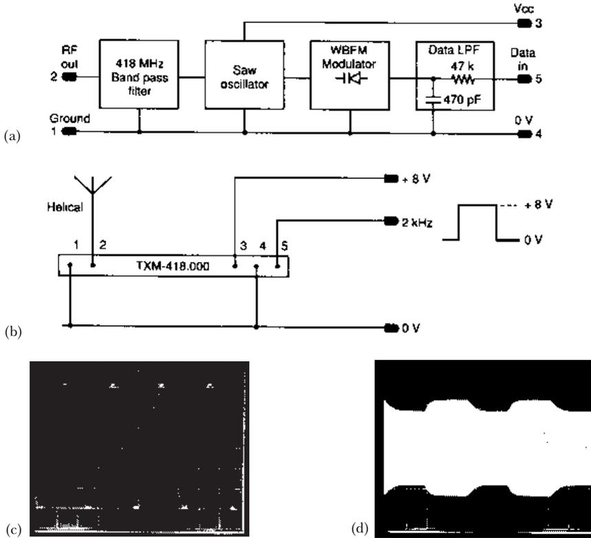
**Figure 7.15** (a) Block diagram of the TX-UHF transmitter module. (b) Connections in recommended test circuit. (c) The output of the transmitter module following 20 dB of attenuation, 10 mV/div. vertical, 1 ns/div. horizontal, 12 V supply, no modulation. (d) As (c) except 9 V supply, 100 μs/div. horizontal, 2.4 kHz squarewave modulation applied
