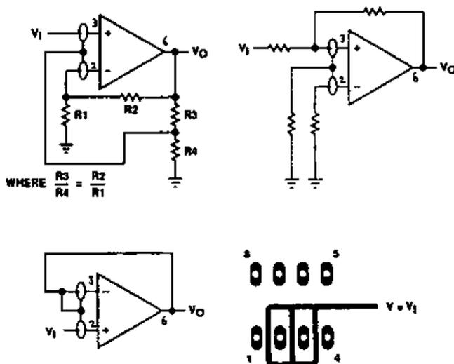
**Figure 3.15** Guard rings around the input terminals minimise the effect of board leakage and capacitance by surrounding the input pins with copper track at the same potential as the input. There is thus no potential difference to force current through any leakage paths or through stray capacitance
