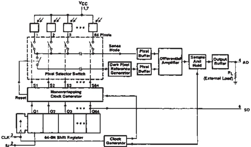
**Figure 5.1** The TSL214 64 element line sensor. The charge stored in each of the 64 pixels during each integration period is read out sequentially via a 64 way mux controlled by the shift register. The charge accumulated in an integration period is proportional to the intensity of the light and the length of the integration period
