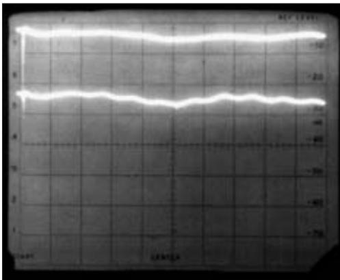
**Figure 3.32** (a) Circuit diagram of a wideband FET input probe with a gain of  $\times 0.5$ . (b) Roughly level output of a sweeper used to test the probe circuit of (a) (upper trace) and output of probe (lower trace). Span 0–1000 MHz, IF bandwidth 1 MHz, 10 dB/div. vertical, ref. level (top of screen) +10 dBm
