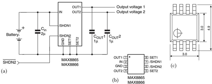
**Figure 1.32** The MAX8865x dual low dropout regulator (a) from MAXIM comes in the proprietary *muMAX* package, with pinout as at (b). At 3 mm, the package length (c) is similar to TSSOP, but the width across pins is 1.5 mm less, which could lead to its more widespread adoption by other manufacturers
