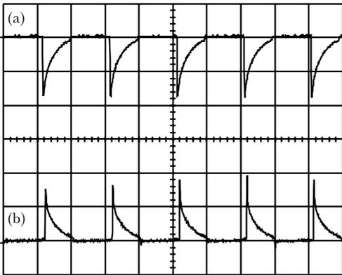
**Figure 5.31** Performance of the circuit of Figure 5.29, continued: (a) lightmeter output (upper trace), 1 V/div. vertical, 0 V line at three divisions above centreline, 10  $\mu$ s/div. horizontal; (b) diode current waveform (monitored across a 0.18  $\Omega$  resistor, lower trace), 50 mV/div. vertical, 0 V line at three divisions below centreline, 10  $\mu$ s/div. horizontal
