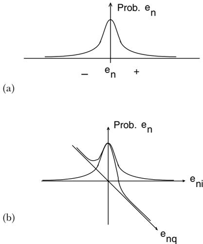
**Figure 7.28** (a) Voltage probability distribution of a real signal (same as Figure 7.24). (b) Voltage probability distribution of the in-phase and quadrature components of a narrowband noise (a complex signal)
