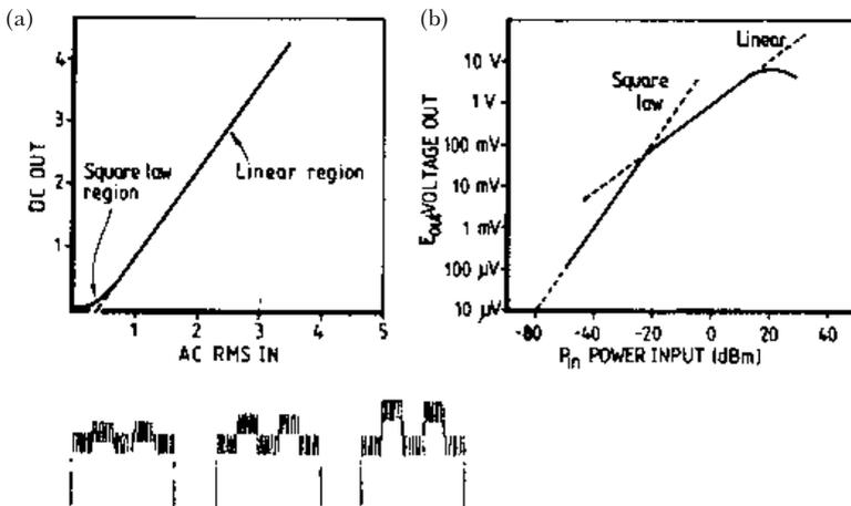
**Figure 4.2** The detection efficiency of the diode detector falls sharply at low signal levels within the square-law region of the diode's response, as the two graphics show. A squarewave modulated carrier can be used to determine sensitivity (see text)
