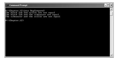
Figure 12-17 Output of the DogCompare2 program when Dog2 overrides equals()
