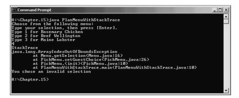
Figure 15-17 Exceptional run of the PlanMenuWithStackTrace program
