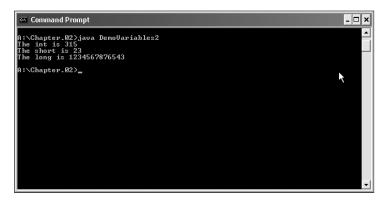
Figure 2-2 Output of the DemoVariables2 program
