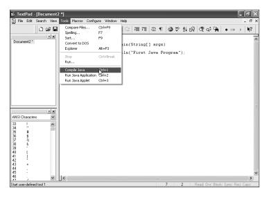
Figure A1-6 Compiling source code using the Tools Menu
