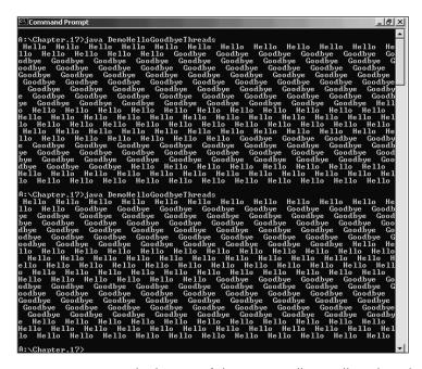
**Figure 17-10** Multiple runs of the DemoHelloGoodbyeThreads program
