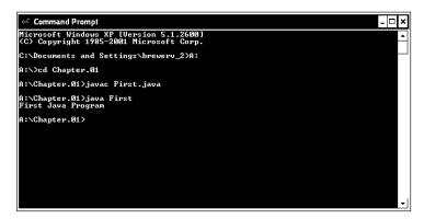
Figure A1-3 Commands for compiling and running the First.java program
