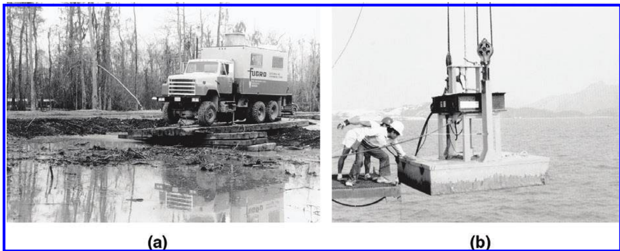
FIGURE 5.4 CPT sounding methods. (a) On land; (b) over water.
