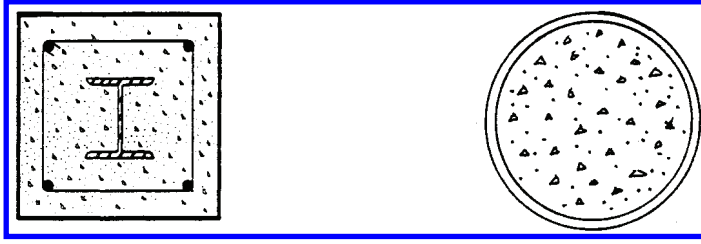
FIGURE 2.11 Typical cross sections of composite columns.
