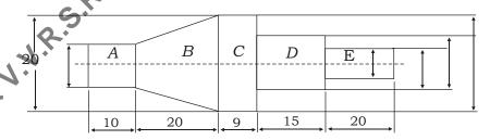
**16.** Find the time required to turn 3.5 cm dia bar to the dimensions shown in the figure. Cutting speed is 17.6 m/min and feed is 1 mm/rev. All cuts are 3.5 mm deep. All dimensions are in mm.
