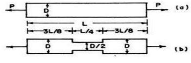
HWA DIST, A.P strain energies of the two bars if the ratio of their modulus of elasticities is 4/7 (E<sub>1</sub>/E<sub>2</sub> = 4/7).
