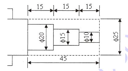
Working Materials: Mild steel, work size: 30 mm dia, Length: 50 mm dia, cutting speed = 600 r.p.m., feed = 150 mm/min, depth of cut should not exceed 2 mm.
