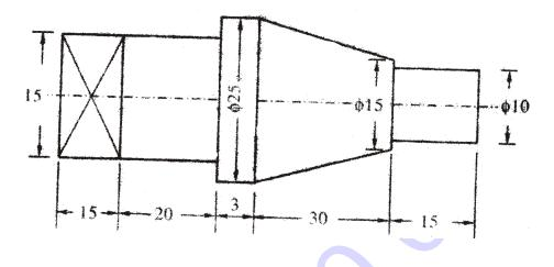
14. The shaft shown below is to be manufactured by turning out of 85 mm steel rod. Find out the minimum machining time if the job is to be turned at 300 r.p.m. with feed 0.5 mm/rev and depth of cut 3 mm. All dimensions are in mm :
