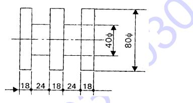
**15.** A product shown in figure below is to be turned from 35 mm diameter and 150 mm long MS bar stock. Calculate the machining time required if depth of cut is not to exceed 5 mm and cutting speed is 20 m/min. Feed is 1 mm/rev. for drilling and facing. Feed for turning is 2 mm/rev.
