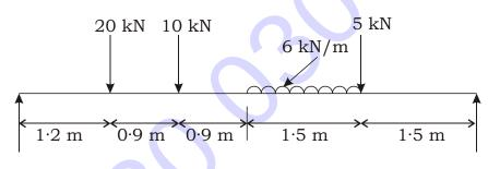
**15.** Draw shear force and bending moment diagram of given cantilever beam :
