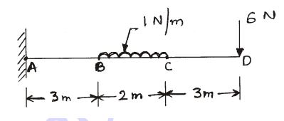
**15.** Draw shear force and bending moment diagrams for a simply supported beam shown in the figure below :
