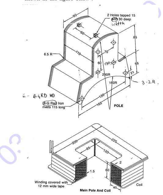
Draw the assembled sectional elevation and plan.
