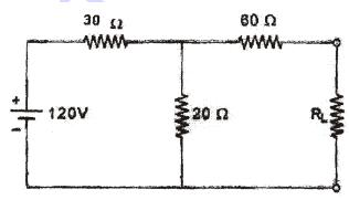
(b) Using Norton's theorem, find the current in the load resistance  $R_L$  of the circuit shown below.
