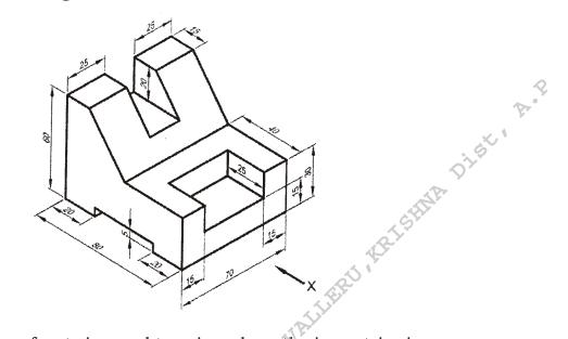
**9.** From the given front view and top view, draw the isometric view :
