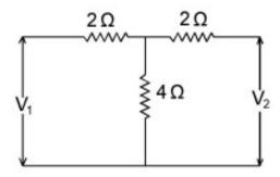
(b) Find the Y-parameters for a given T-network (6M)
