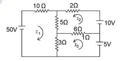
\*13) Determine the voltages  $V_1$  in the given network using nodal voltage analysis?.
