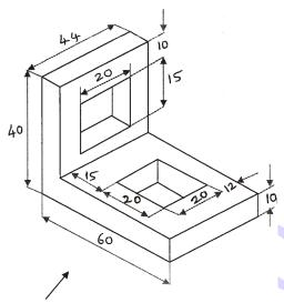
**9.** Draw the isometric drawing of an object whose orthographic projections are given below:
