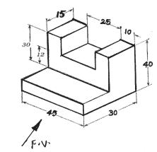
**8.** Draw the sectional front view, top view and side view of the object shown below.
