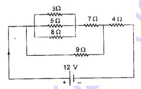
**12.** Find the equivalent resistance the between points A and B of the circuit shown using star/delta transformation :
