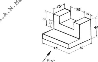
**8.** Draw the sectional front view, top view and side view of the object shown below.
