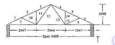
Tie beam : 2 nos. back to back ISA 50 mm  $\times$  50 mm  $\times$  6 mm @ 4-5 kg/m
