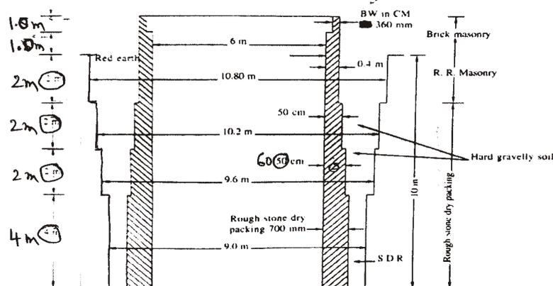
18. Calculate the quantities of the following items of a septic tank as shown in figure :
