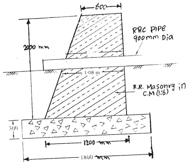
9. The cross-section of a soak pit of 1.8 m dia is shown in figure. Calculate the earthwork excavation for soak pit :
