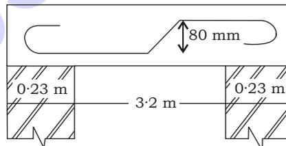
3. Calculate the number of stirrups of 8 mm dia for a simply supported beam of size 200 mm × 350 mm. Spacing of stirrups is 200 mm centre to centre, total length of beam is 5.8 m. Assume end cover of 25 mm.
