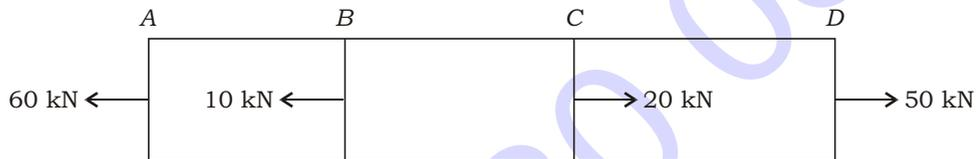
Find the change in length of the bar.  $E = 200 \text{ kN/mm}^2$ ,  $AB = 600 \text{ mm}$ ,  $BC = 700 \text{ mm}$  and  $CD = 800 \text{ mm}$ .
