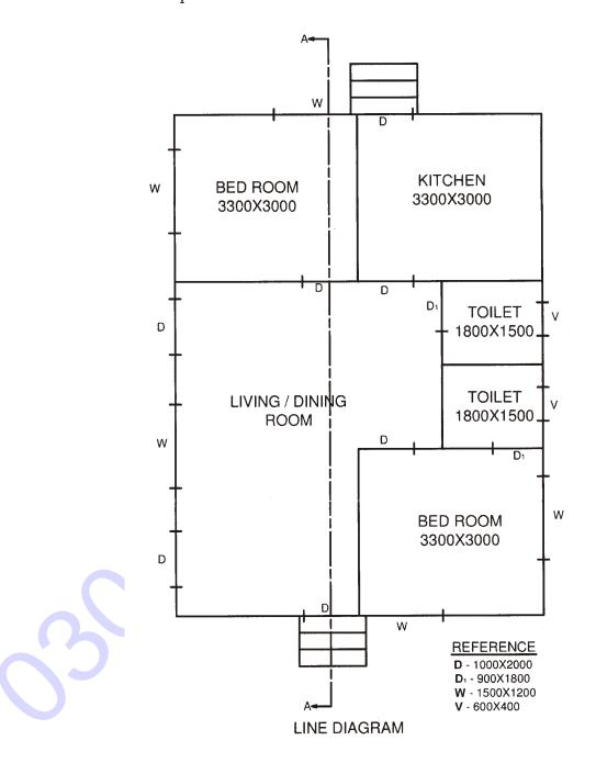
(iv) Superstructure: All the walls are 200 mm thick except partition wall between toilets which is constructed on the floor with thickness of 100 mm. The height of walls is 3300 mm to the bottom of RCC roof slab.
