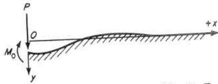
Fig. 4.5. Semi-infinite Beam on an Elastic Foundation
