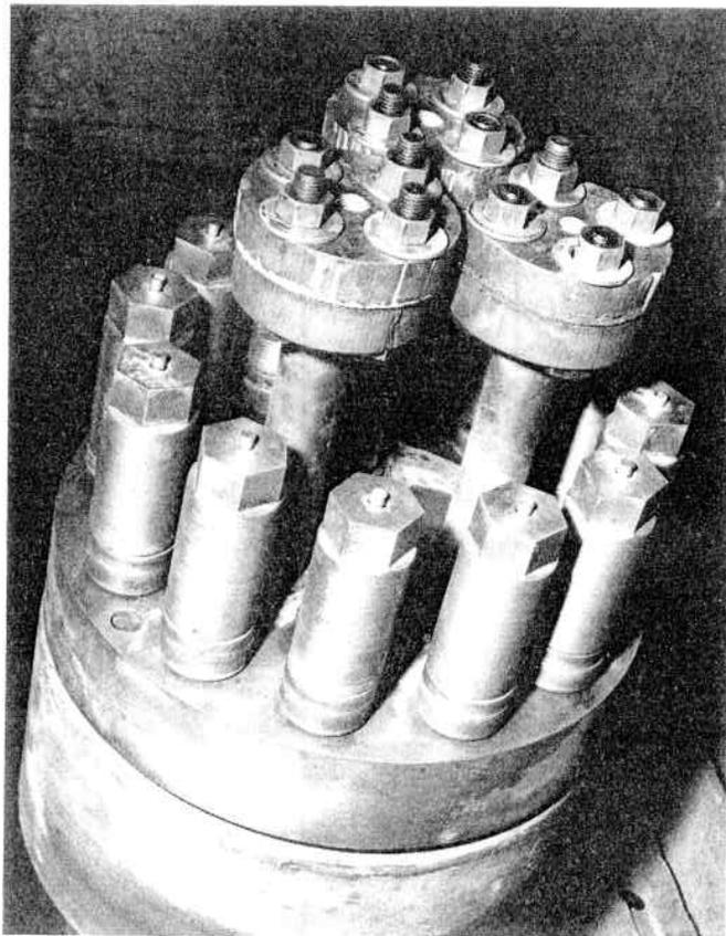
Fig. 6.40. Pressure Vessel Flange Showing the Use of Sleeve Type Nuts and Spherical Washers for the large Studs, and Conventional Nuts and Flat Washers for the Small Studs. The Rods Protruding Through the Nuts Extend Through a Central Stud Hole for the Purpose of Measuring Stud Elongation and Stresses
