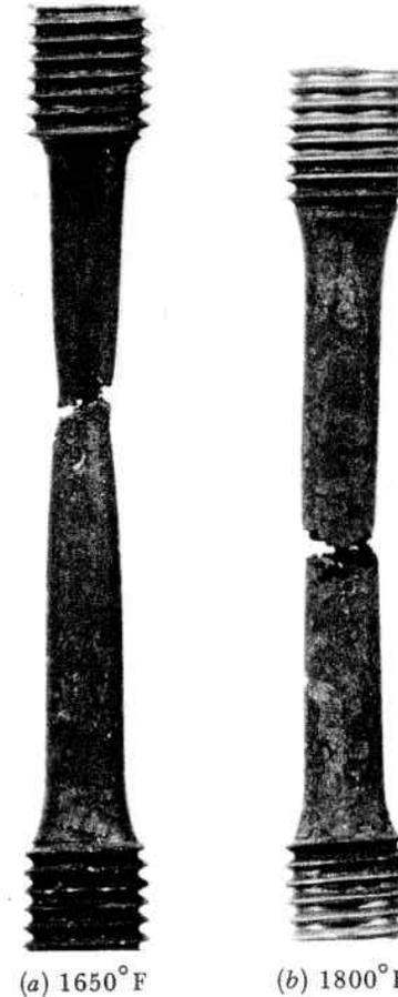
Fig. 5.73. Nature of Ductility Loss at High Elevated Temperatures, Mild Carbon Steel. Specimens Were of the Same Material and Initially the Same Length.
