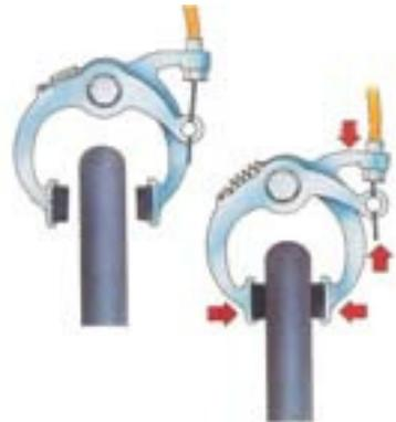
When brakes are on, the pads grip the wheel rim from either side, friction between the pads and the rim converts the cycle's kinetic energy into heat as they reduce its speed.
