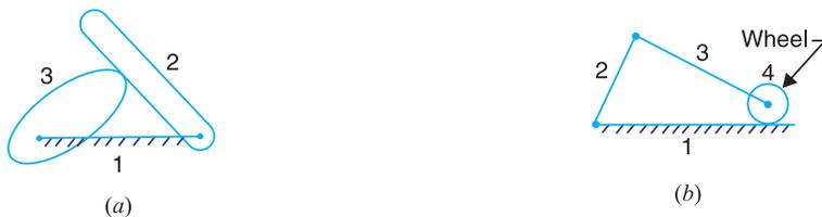
Fig. 5.17. Mechanism with a higher pair.
