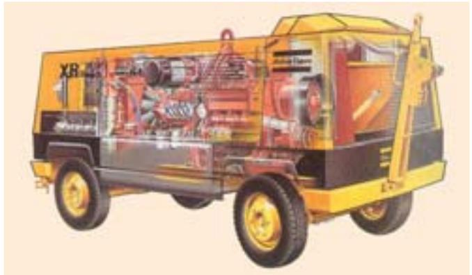
This industrial compressor uses compressed air to power heavy-duty construction tools. Compressors are used for jobs, such as breaking up concrete or paving, drilling, pile driving, sand-blasting and tunnelling. A compressor works on the same principle as a pump. A piston moves backwards and forwards inside a hollow cylinder, which compresses the air and forces it into a hollow chamber. A pipe or hose connected to the chamber channels the compressed air to the tools.
