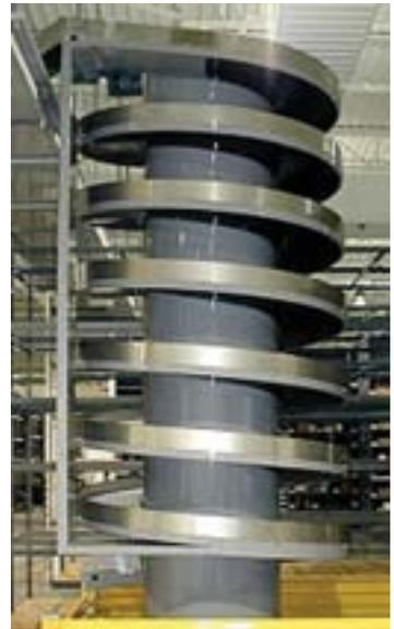
A spiral elevator conveyor for material handling.
