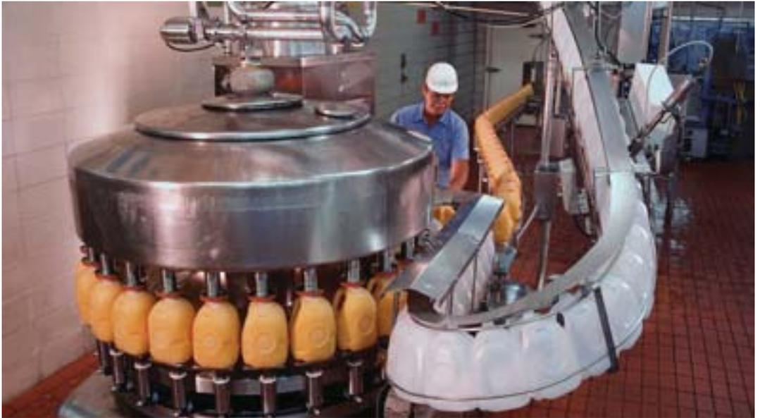
An automatic filling and sealing machine.
