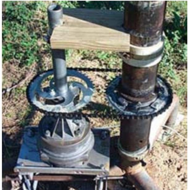
The chains are mostly used to transmit motion and power from one shaft to another, when the distance between the centres of the shafts is short such as in bicycles, motor cycles, agricultural machinery, road rollers, etc.
