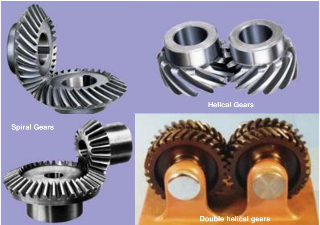
**3. According to the type of gearing.** The gears, according to the type of gearing may be classified as :
