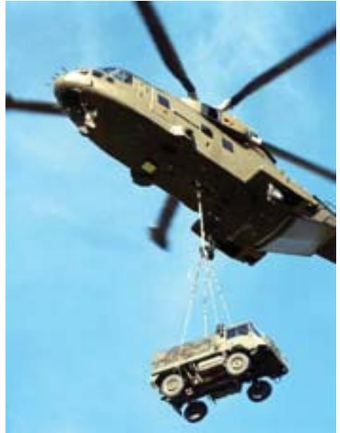
Blades of the helicopter propeller push the air downwards and the resultant reaction gives helicopter the necessary lifting power.
