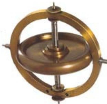
Gyroscopic inertia prevents a spinning top from falling sideways.
