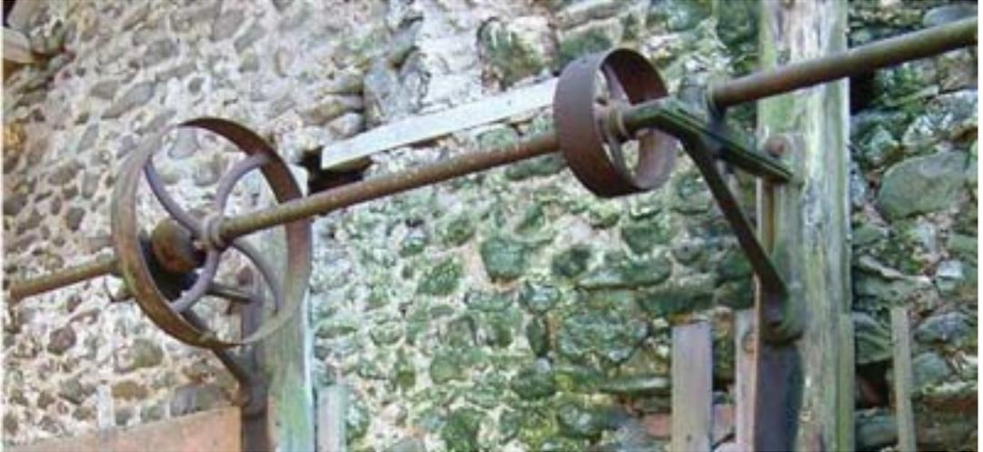
When loads are applied on the above two pulleys, the shaft is subject to torsional vibration
