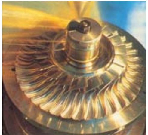
Nowadays steam turbines like this can be produced entirely by computer-controlled machine tools, directly from the engineer's computer.
