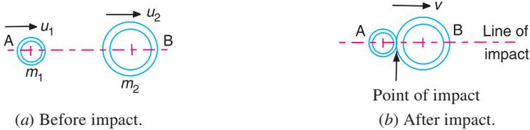
**Fig. 3.16.** Collision of inelastic bodies.
