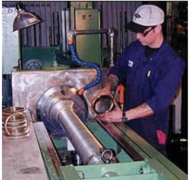
**Broaching machine.** Broaching is a process of machining through holes of any cross sectional shape, straight and helical slots, external surfaces of various shapes, external and internal toothed gears, splines, keyways and rifling.
