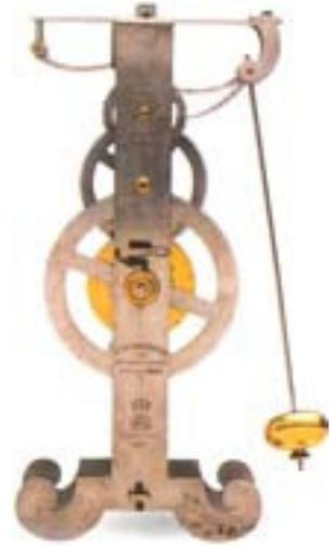
A pendulum clock designed by Galileo. Galileo was the first to design a clock based on the relationship between gravitational force ( $g$ ), length of the pendulum ( $l$ ) and time of oscillation ( $t$ ).
