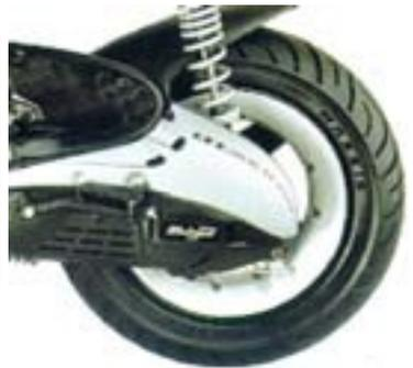
Helical spring suspension of a two-wheeler.
