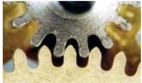
Let the wheel  $A$  be keyed to the rotating shaft and the wheel  $B$  to the shaft, to be rotated. A little consideration will show, that when the wheel  $A$  is rotated by a rotating shaft, it will rotate the wheel  $B$  in the opposite direction as shown in Fig. 12.1 (a).
