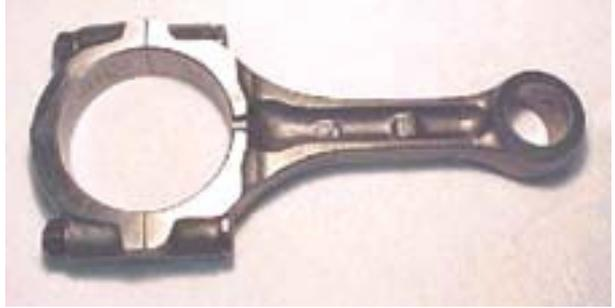
Connecting rod of a petrol engine.
