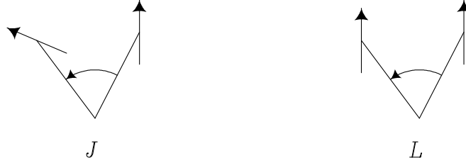
Figure 7.3 J both swings the particle around the origin and rotates its spin (left), while L moves the particle, but leaves the direction of the spin invariant (right).
