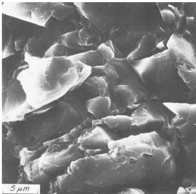
**Figure 4.9** Magnification of “smooth” fracture surface of quartz.
