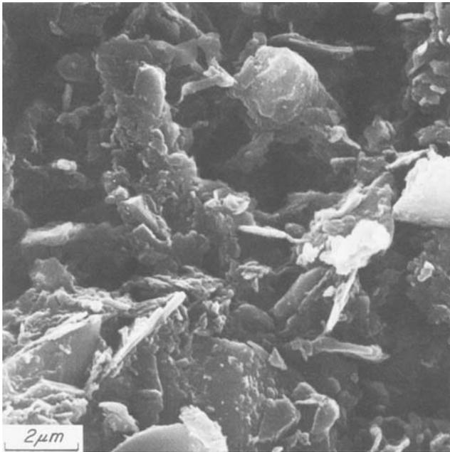
**Figure 4.12** Fabric of undisturbed Berthierville clay.
