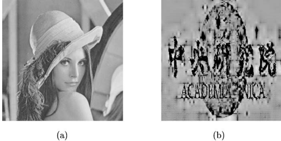
FIGURE 18.11 Jitter attack [four pairs of columns, (90, 200), (50, 150), (120, 110), and (1, 3), were deleted/duplicated]. (a) Jitter-attacked watermarked image; (b) retrieved watermark.
