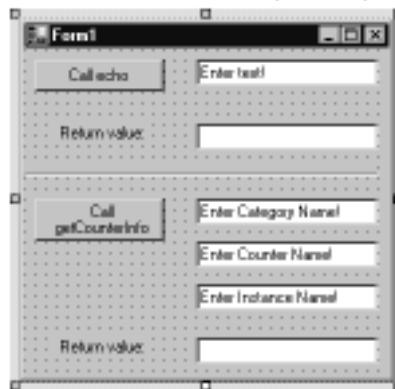
Figure 11.47 Adding Elements on the Windows Form for the getCounterInfo method (Form1.cs in soapExamplesClient )
