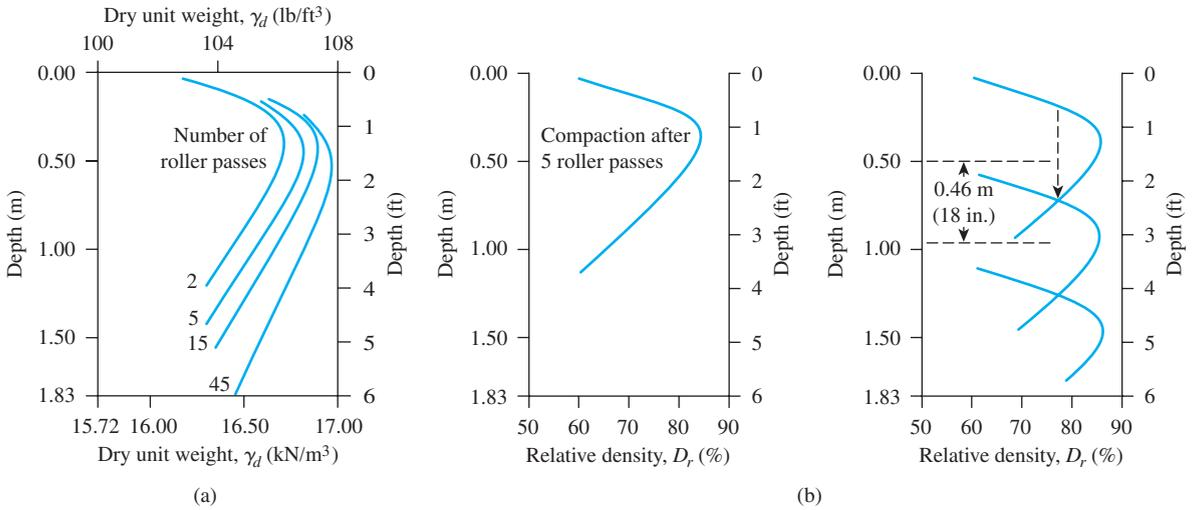
**Figure 6.20** (a) Vibratory compaction of a sand—variation of dry unit weight with number of roller passes; thickness of lift = 2.44 m (8 ft); (b) estimation of compaction lift thickness for minimum required relative density of 75% with five roller passes (After D'Appolonia, Whitman, and D'Appolonia, 1969. With permission from ASCE.)
