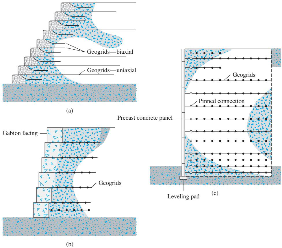
**Figure 13.37** Typical schematic diagrams of retaining walls with geogrid reinforcement: (a) geogrid wraparound wall; (b) wall with gabion facing; (c) concrete-panel-faced wall
