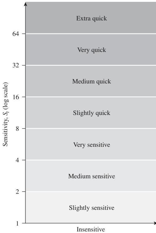
**Figure 12.38** Classification of clays based on sensitivity
