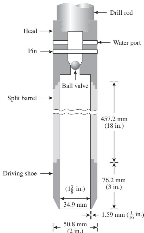
**Figure 18.5** Diagram of standard split- spoon sampler
