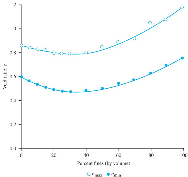
**Figure 3.8** Variation of  $e_{\max}$  and  $e_{\min}$  (for Nevada 50/80 sand) with percentage of non-plastic fines (Redrawn from Lade *et al.*, 1998. Copyright ASTM INTERNATIONAL. Reprinted with permission.)
