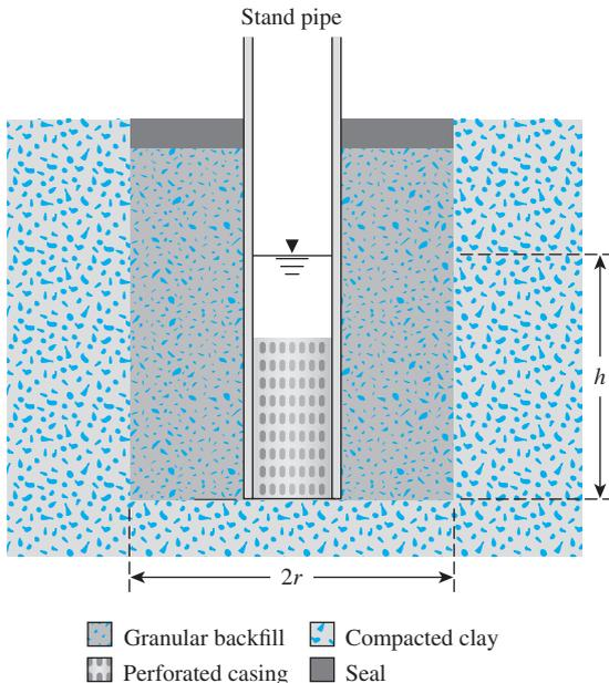
**Figure 7.25** Borehole test with constant water level
