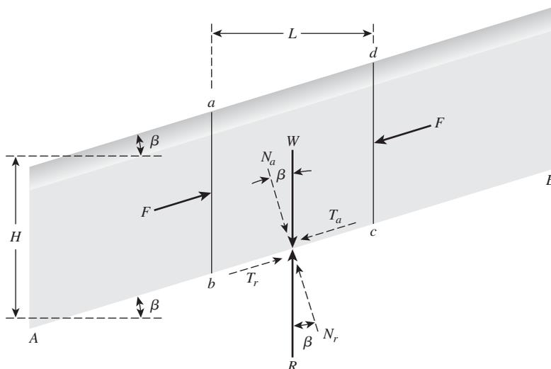
**Figure 15.7** Analysis of infinite slope (without seepage)
