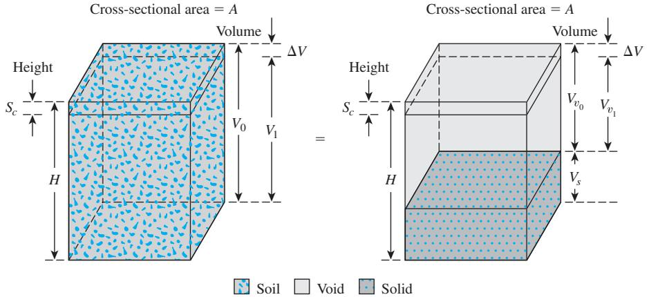
Figure 11.16 Settlement caused by one-dimensional consolidation
