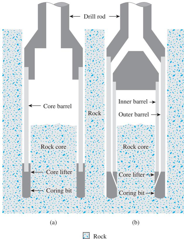
**Figure 18.14** Rock coring: (a) single-tube core barrel; (b) double-tube core barrel
