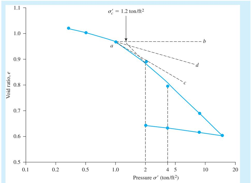
Figure 11.17 Plot of  $e$  versus  $\log \sigma'$
