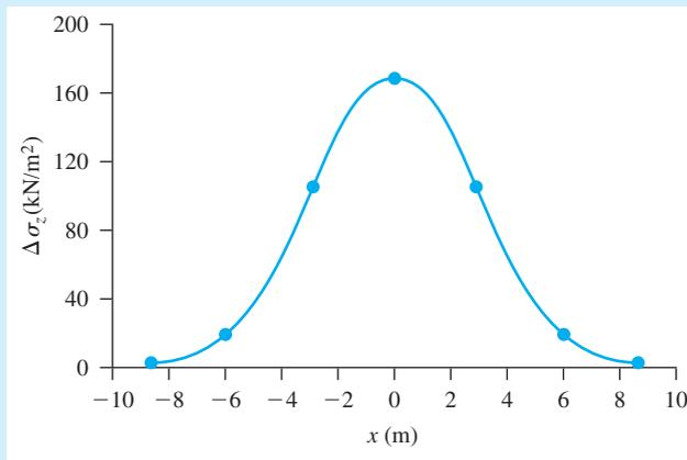
Figure 10.13 Plot of  $\Delta\sigma_z$  against distance  $x$
