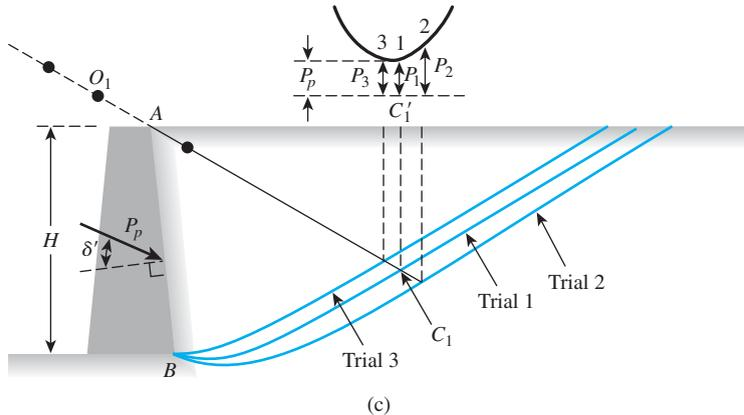
**Figure 14.3** Passive earth pressure against retaining wall with curved failure surface
