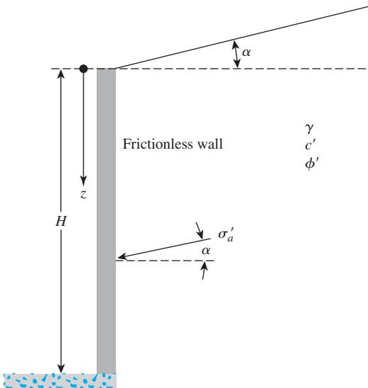
Figure 13.12 Frictionless vertical retaining wall with sloping backfill
