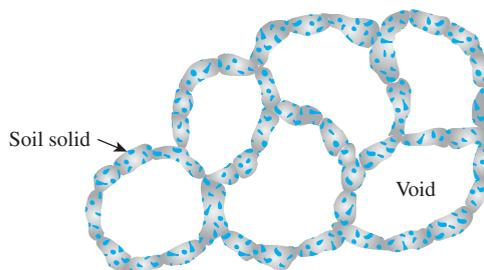
**Figure 4.20** Honeycombed structure
