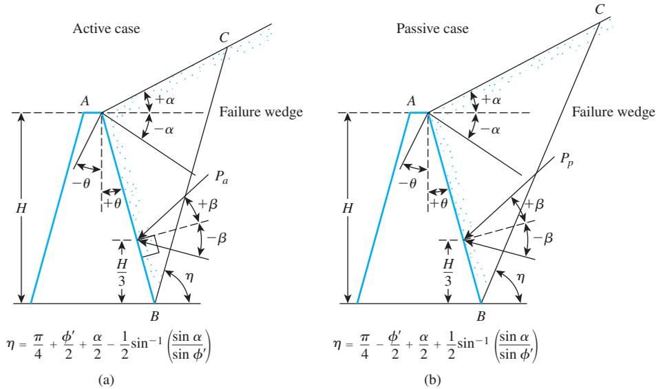
Figure 13.11 Location and direction of resultant Rankine force
