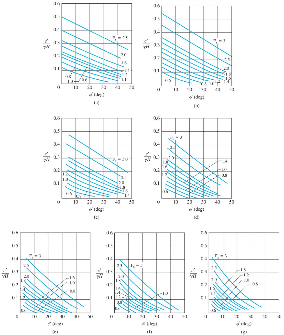
**Figure 15.25** Contours of equal factors of safety: (a) slope – 1 vertical to 0.5 horizontal; (b) slope – 1 vertical to 0.75 horizontal; (c) slope – 1 vertical to 1 horizontal; (d) slope – 1 vertical to 1.5 horizontal; (e) slope – 1 vertical to 2 horizontal; (f) slope – 1 vertical to 2.5 horizontal; (g) slope – 1 vertical to 3 horizontal (After Singh, 1970. With permission from ASCE.)
