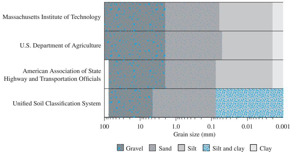
**Figure 2.7** Soil-separate-size limits by various systems
