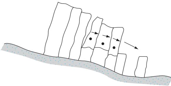
**Figure 15.3** Slope failure by “toppling”
