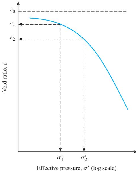
Figure 11.10 Typical plot of  $e$  against  $\log \sigma'$
