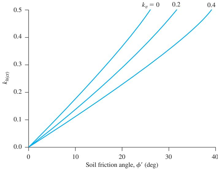
**Figure 13.28** Critical values of horizontal acceleration (Eq. 13.90)
