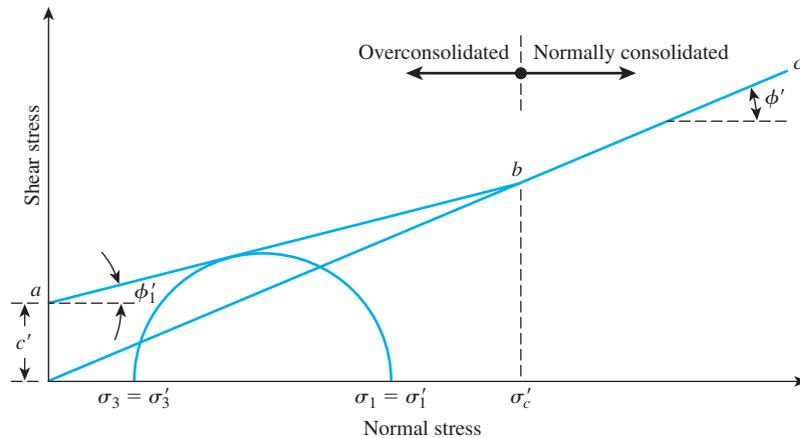
Figure 12.23 Effective stress failure envelope for overconsolidated clay
