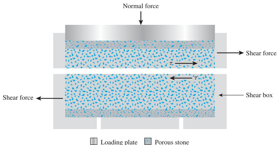
**Figure 12.4** Diagram of direct shear test arrangement
