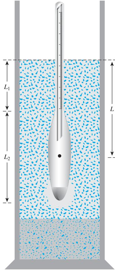
**Figure 2.24** Definition of  $L$  in hydrometer test
