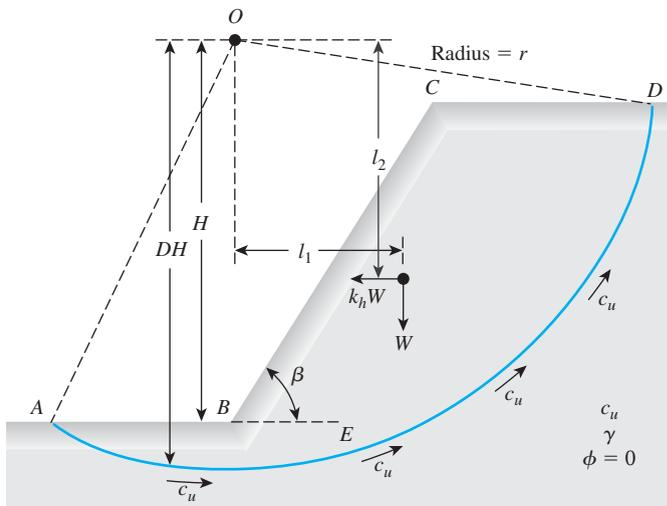
**Figure 15.18** Stability analysis of slope in homogeneous saturated clay with earthquake forces ( $\phi = 0$  condition)
