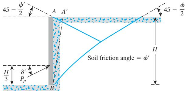
**Figure 14.1** Effect of wall friction on failure surface
