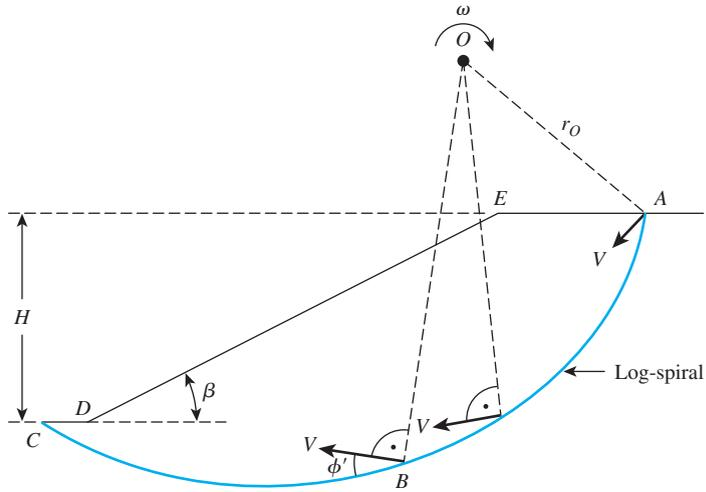
**Figure 15.26** Stability analysis using rotational collapse mechanism
