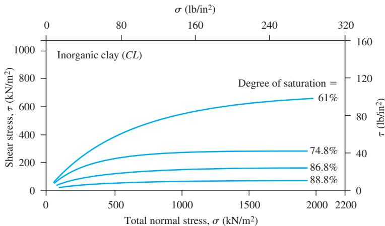
**Figure 12.52** Variation of the total stress failure envelope with change of initial degree of saturation obtained from undrained tests of an inorganic clay (After Casagrande and Hirschfeld, 1960. With permission from ASCE.)
