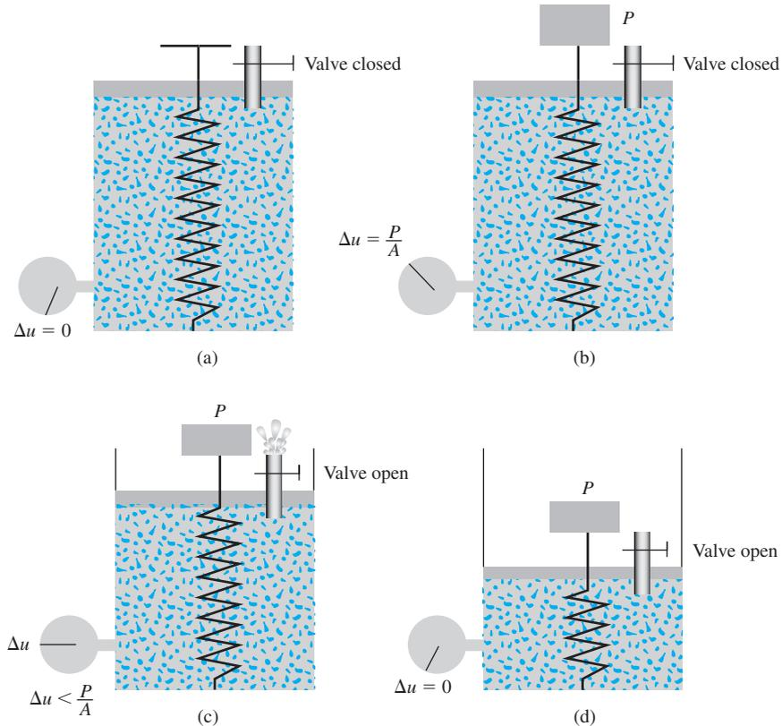
Figure 11.5 Spring-cylinder model
