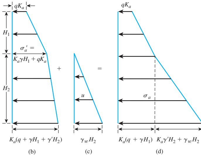
**Figure 13.14** Rankine's active earth-pressure distribution against a retaining wall with partially submerged cohesionless soil backfill supporting a surcharge
