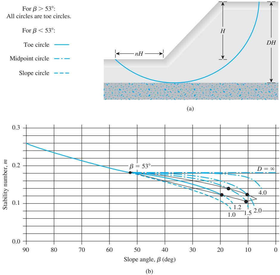
**Figure 15.13** (a) Definition of parameters for midpoint circle type of failure; (b) plot of stability number against slope angle (Adapted from Terzaghi and Peck, 1967. With permission of John Wiley & Sons, Inc.)
