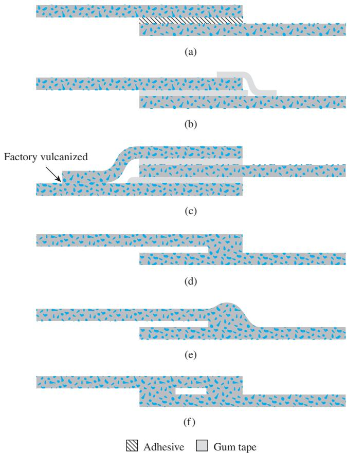
**Figure 17.6** Configurations of field geomembrane seams: (a) lap seam; (b) lap seam with gum tape; (c) tongue-and-groove splice; (d) extrusion weld lap seam; (e) fillet weld lap seam; (f) double hot air or wedge seam (After U.S. Environmental Protection Agency, 1989)
