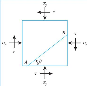
**Figure 10.4** Soil element with stresses acting on it
