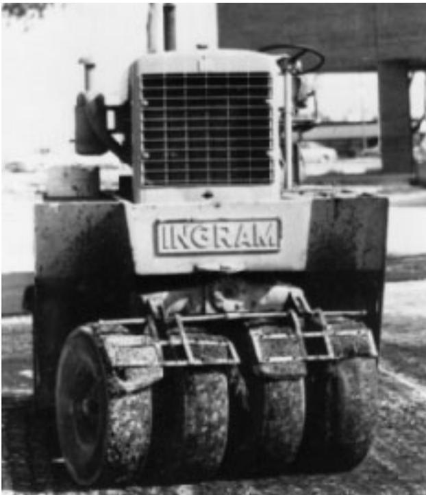
**Figure 6.16** Pneumatic rubber-tired roller (*Ingram Compaction LLC*)
