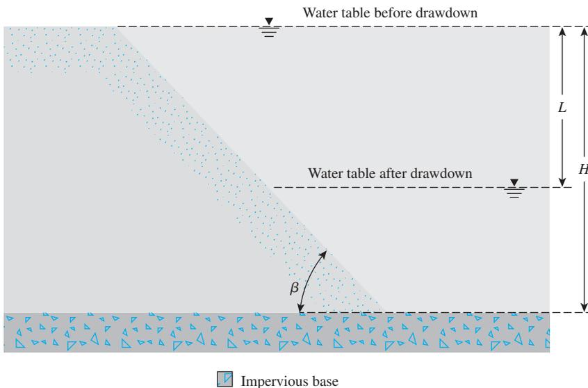
Figure 15.41 Stability analysis for rapid drawdown condition
