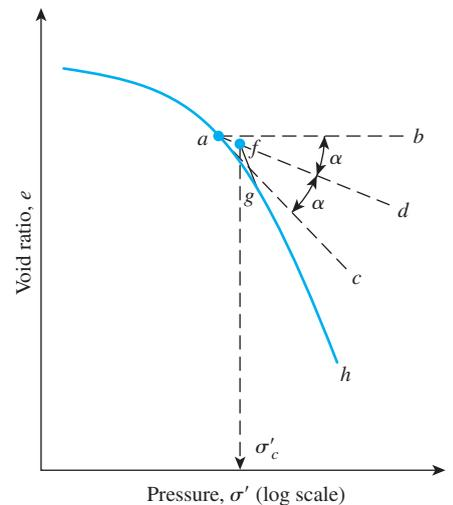
**Figure 11.13** Graphic procedure for determining preconsolidation pressure
