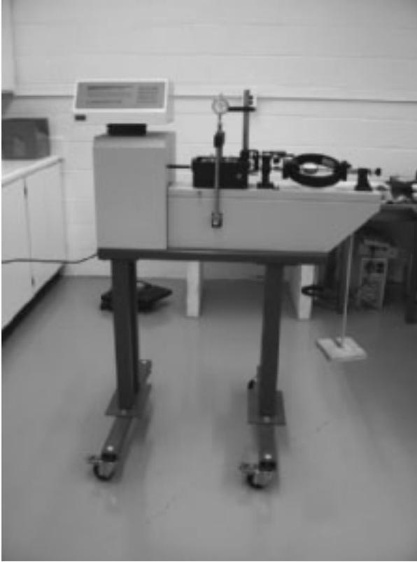
**Figure 12.5** Strain-controlled direct shear equipment
