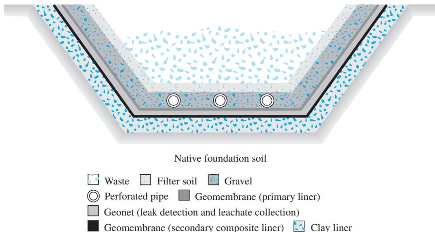
**Figure 17.10** Cross section of double-liner system (note the secondary composite liner)
