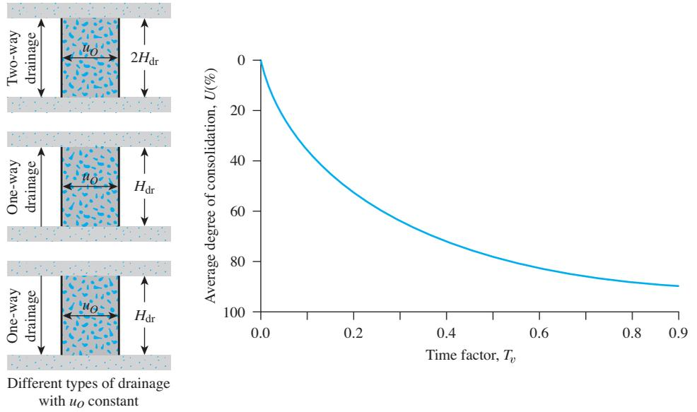
**Figure 11.24** Variation of average degree of consolidation with time factor,  $T_v$  ( $u_0$  constant with depth)
