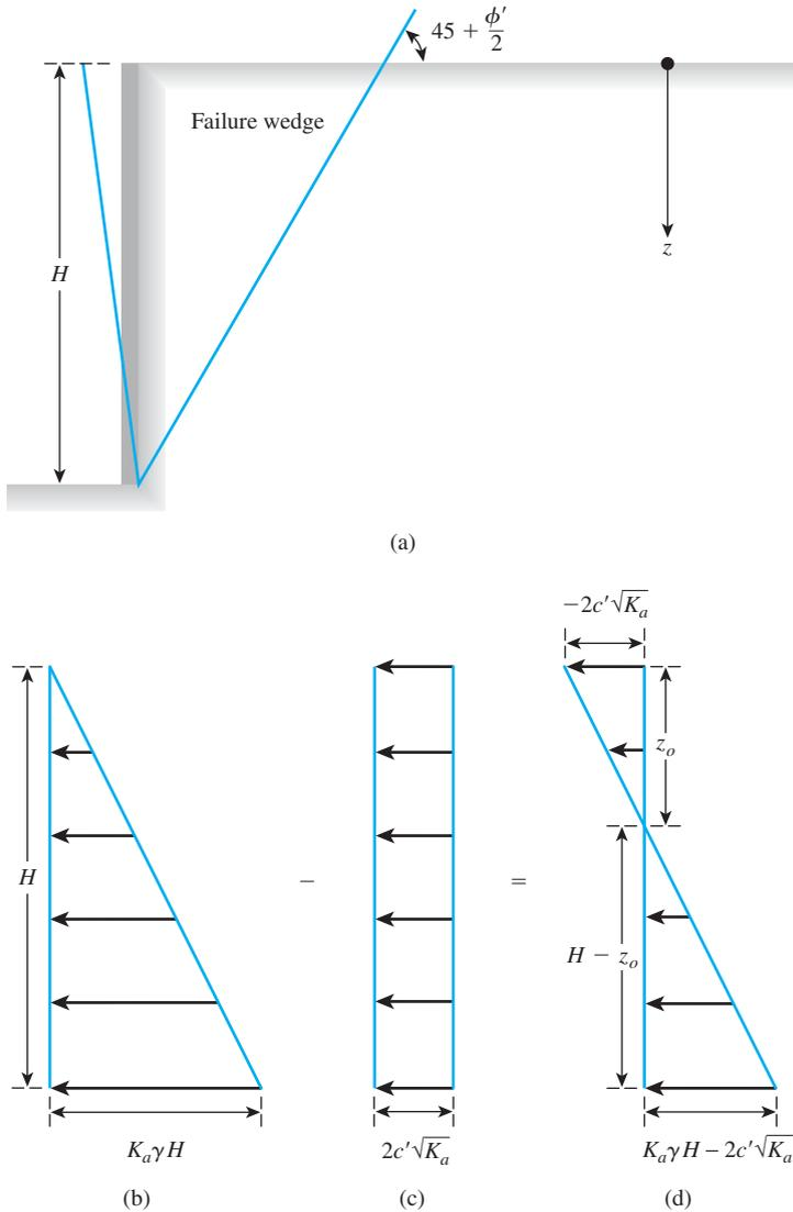
**Figure 13.16** Rankine's active earth-pressure distribution against a retaining wall with cohesive soil backfill
