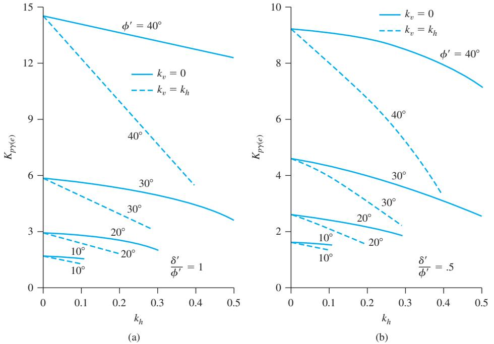
**Figure 14.6** Variation of  $K_{p\gamma(e)}$ : (a)  $\delta'/\phi' = 1$ ; (b)  $\frac{\delta'}{\phi'} = 0.5$
