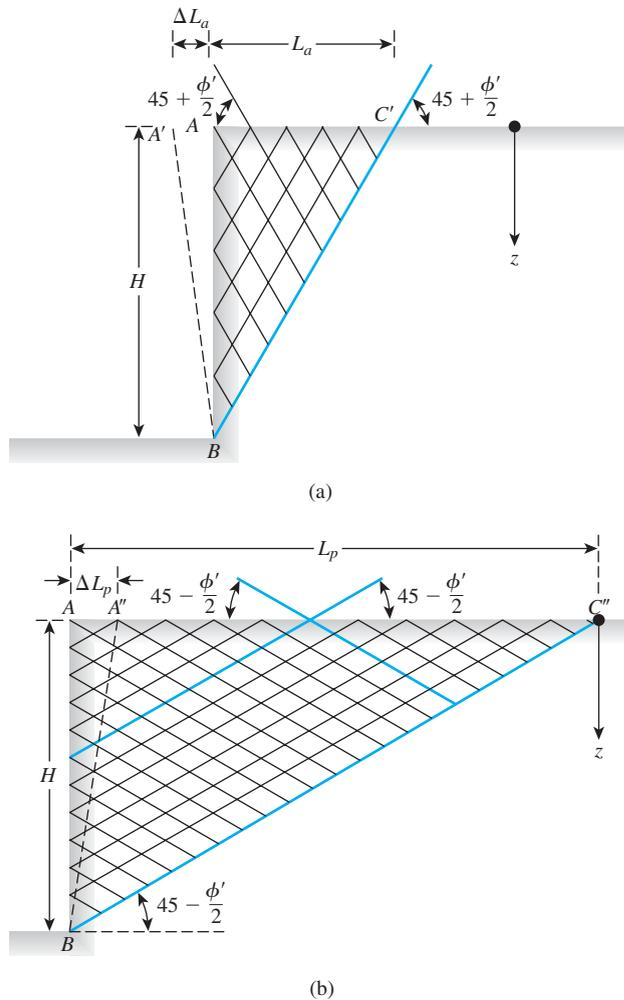
**Figure 13.9** Rotation of frictionless wall about the bottom
