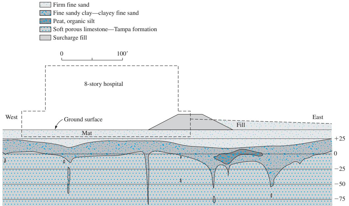
**Figure 11.31** Simplified general subsoil conditions at the site of Tampa VA Hospital (After Wheelen and Sowers, 1972. With permission from ASCE.)
