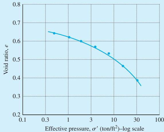
Figure 11.11 Variation of void ratio with effective pressure
