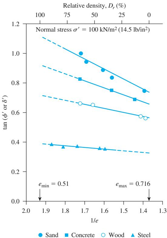
**Figure 12.15** Variation of  $\tan \phi'$  and  $\tan \delta'$  with  $1/e$  [Note:  $e$  = void ratio,  $\sigma' = 100 \text{ kN/m}^2$  (14.5 lb/in.<sup>2</sup>), quartz sand] (After Acar, Durgunoglu, and Tumay, 1982. With permission from ASCE.)
