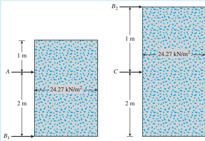
**Figure 14.14** Calculation of strut loads from pressure envelope
