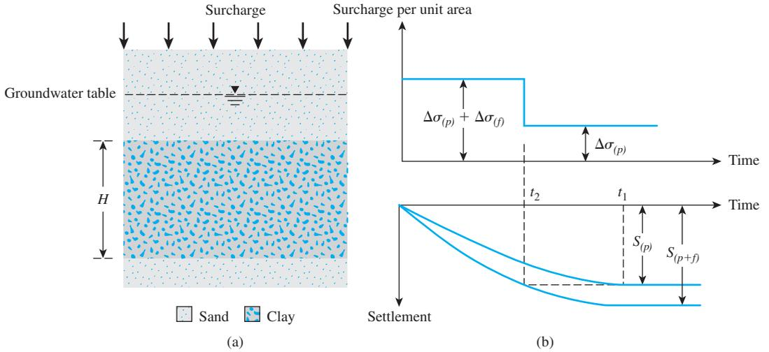
**Figure 11.39** Principles of precompression
