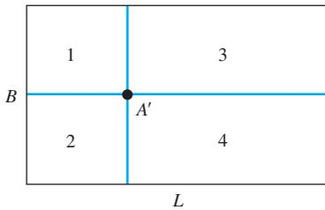
**Figure 10.22** Increase of stress at any point below a rectangularly loaded flexible area
