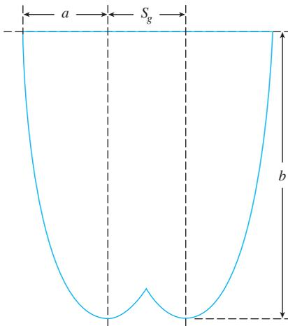
**Figure 6.37** Approximate grid spacing for dynamic compaction
