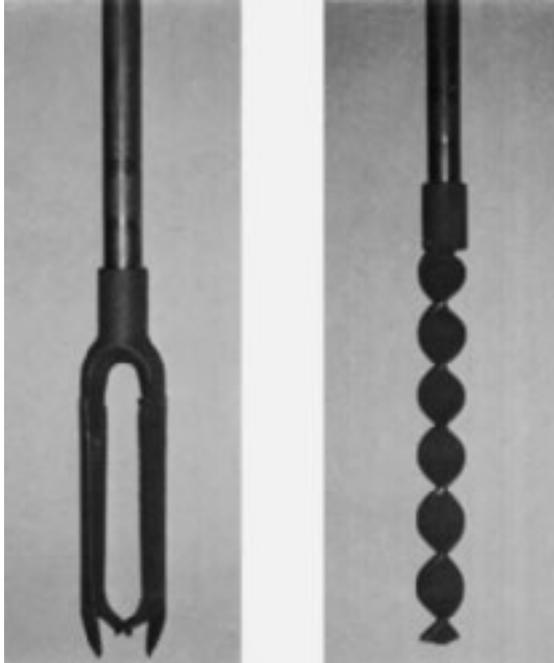
**Figure 18.1** Hand augers: (a) Iwan auger; (b) slip auger
