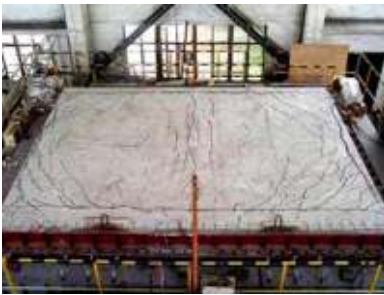
Fig. 9.23 Cracks on the S-2 after the test
