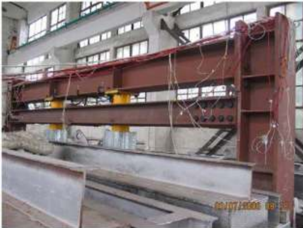
Fig. 7.6 Full view of the test set-up
