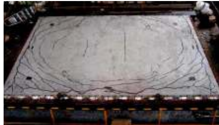
Fig. 9.27 Cracks on S-4 after the test
