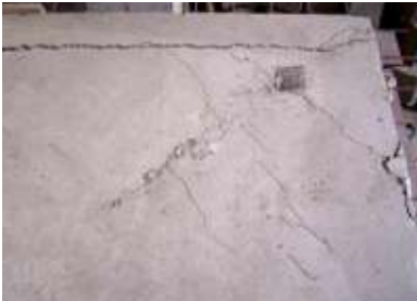
Fig. 9.21 Yield lines at the corner on S-1
