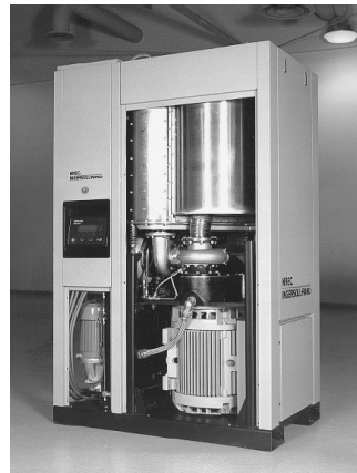
FIGURE 5.19 Highly recuperated, two-shaft microturbine. (Courtesy of Ingersoll-Rand Energy Systems, with permission.)
