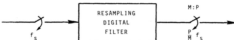
Fig. 3.14. Input and output rates of resampling digital filter.
