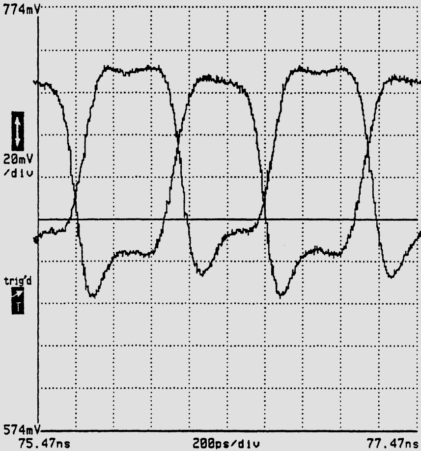
Figure 7.21 The measured output waveforms of the new receiver test structure at 1 GHz with 4V input signal termination (attenuation at the sampling scope inputs is 20db).
