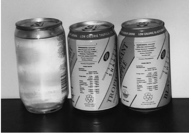
FIGURE 8.5 An example of the competition between materials. The beverage can body can be made of aluminum ( right ), steel ( middle ), and plastic ( left ).
