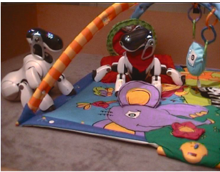
Fig. 3. The robot, placed on a play mat, can move its arms, its neck and mouth and produce sounds. Various toys are placed near the robot, as well as a pre-programmed “adult” robot which can respond vocally to the other robot in certain conditions. Results obtained after a typical run of the experiment are shown. Top curves: relative frequency of the use of different actuators (head pan/tilt, arm, mouth, sound speaker). Bottom curves: frequency of looking towards each object and in particular towards the “adult” pre-programmed robot.
