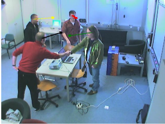
Fig. 5. Estimating Head Pose and Focus of Attention [9]. Head orientations are estimated from four camera views. These are then mapped to likely focus of attention targets, such as room occupants.
