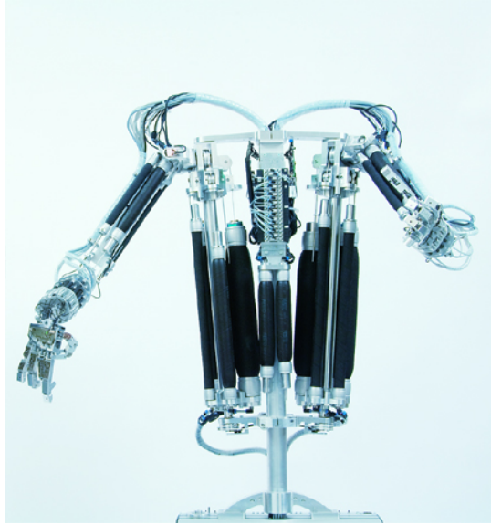
Fig. 2. The humanoid robot torso ZAR5 with two arms and two five-finger hands
