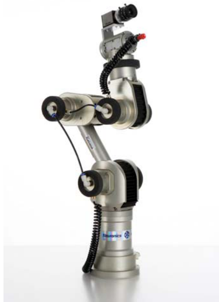
Fig. 1. Katana robot with vacuum gripper and high-resolution camera system placed near the end effector
