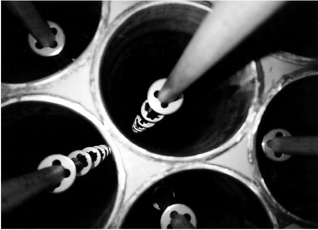
FIGURE 24.1 Tubular collection electrode. (Courtesy of Geoenergy International, Inc.)
