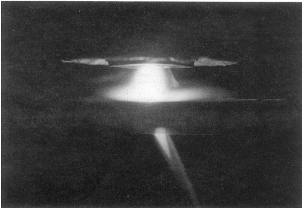
Figure 10.45 Formation of the keyhole and efflux plasma in plasma keyhole welding of 5.0 mm stainless steel. The efflux plasma is inclined backwards as the arc cuts through the plate
