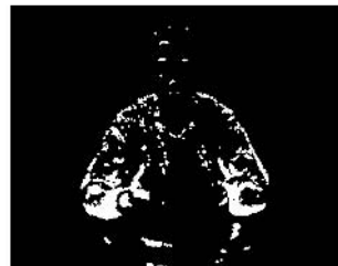
Figure 18: Initial motion mask (after pixel difference thresholded to 10% of max.).
