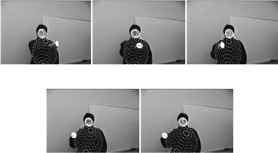
Figure 11. Example ellipsoids for “pointing camera1” activity from front and side view.
