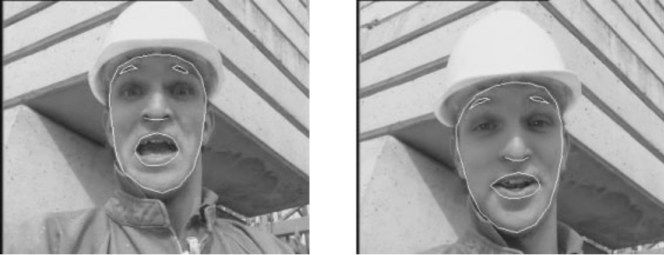
Figure 4. By using snakes, face and feature contours are tracked on each frame of the sequence. Images courtesy of the Image Processing Group at the Universitat Politècnica de Catalunya.
