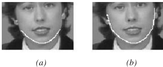
Figure 7. Estimation of chin and cheek contours: (a) Estimated chin contour, (b) Estimated chin and cheek contours.
